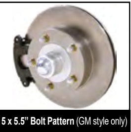
11" with 4 Piston Calipers
