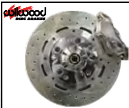
11" with 4 Piston Calipers
