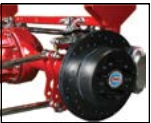
12" Disc w/ Internal Parking Brake
