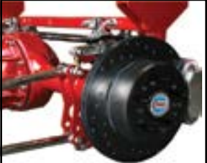
12" Disc w/ Internal Parking Brake
