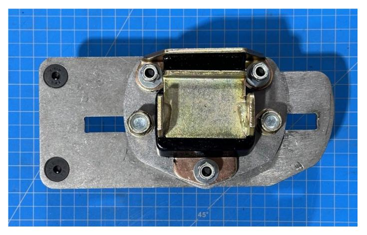
Here is the completed assembly on the passenger side. Set the engine in place, adjust the fore/aft position as needed. When the engine position is correct, tighten the two  $\frac{1}{2}$ " x 13 Nylock nuts on each side. Attach the engine to the chassis using the two  $\frac{7}{16}$ "- 20 x 3.5" bolts, four  $\frac{7}{16}$  flat washers and two  $\frac{7}{16}$ -20 Nylock nuts.
