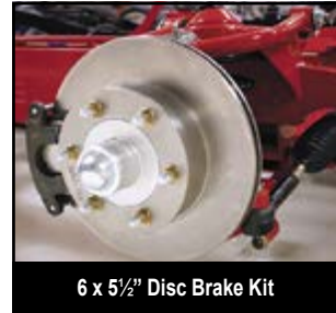
12" Disc w/ Internal Parking Brake
