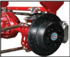
12" Disc w/ Internal Parking Brake
