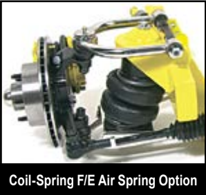
12" Disc w/ Internal Parking Brake
