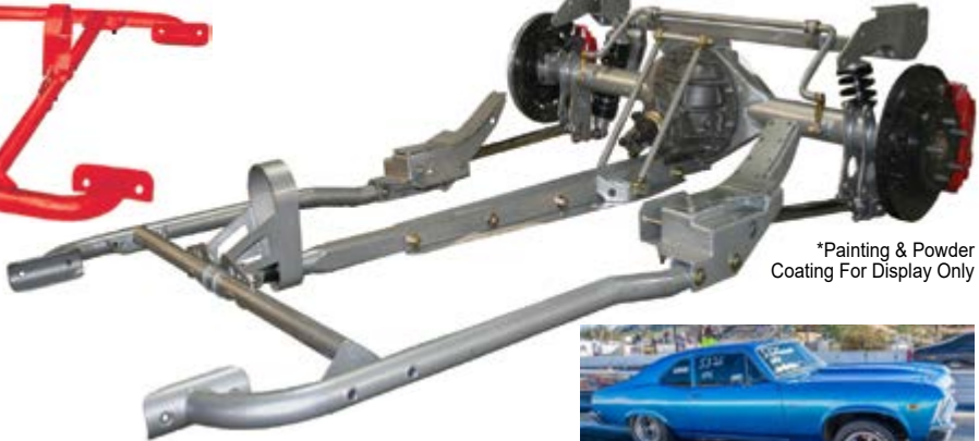
Shown with optional complete rear end, anti-sway bar and RideTech coil-overs.
