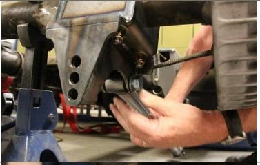
Place the NON adjustable side of the link bar into the bottom of the axle bracket using the provided 5/8" bolt.
