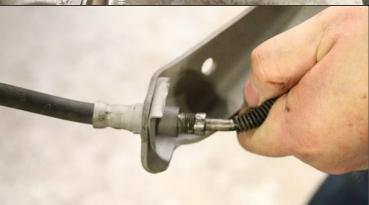
You can now connect the brake line to the brake hose.
