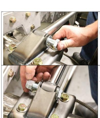
Place the NON adjustable side of the link bar into the top of the axle bracket using the provided 5/8" bolt.
