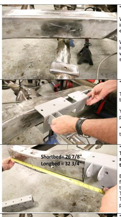
We cleaned up the frame and the housing before installing the new bracketry. We like to mock everything up before any paint is applied.
