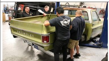
Disconnect wiring, remove bed bolts, disconnect gas fill hose and remove the bed
