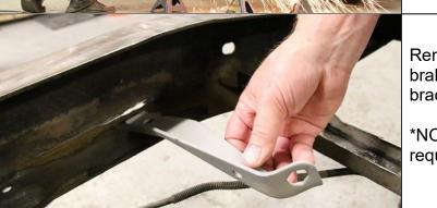
Remove the brake hose and the hard line from the brake line bracket. Then remove the brake line bracket from the frame.
