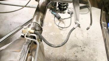
With the bracket installed you can now connect the brake hose and clip from the axle.
