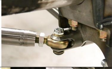
Install the track bar heim joint onto the clevis using the ½" button head bolt. You may have to clock the clevis slightly so the heim doesn't bind. Tighten down the nylock.
