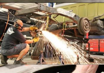
You will need to grind the axle housing smooth where the factory shock mounts used to be.
