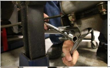
The clevis can be tightened down now. Make sure the flat surfaces are parallel to the ground and each other.
