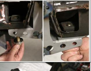
After placing the clip under the original mounting holes install the 2 front mounting bolts (5/8 by 11 by 2 inches long) with the lock washer and the ¼ inch thick by 1.625 washers into the factory cage nuts. The front and rear factory rubber bushings are not used; only the very front core support bushing is used. Leave the bolts finger tight to allow centering the clip.
