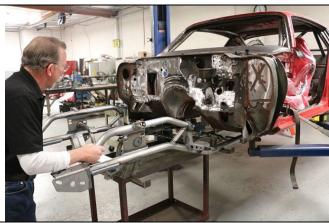
The wheel wells and mounting brackets have to be removed before installing the clip. We chose to remove the whole fender assembly (only 8 bolts). With the fenders on it's difficult to squeeze the clip between the firewall and the front lower valence. When the wheel wells are installed later, they will have to be trimmed on the front edge to clear the outside edge of the top and bottom rail.
