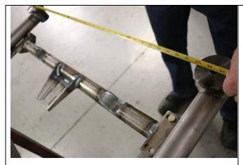
The rear frame rails pull together after the clip is removed from the weld fixture. To facilitate installation and proper alignment, spread the rails and temporarily install the transmission crossmember with the bolt hole centers at 33.5 inch. Once the suspension clip is installed and all bolts tightened, you can remove the crossmember.
