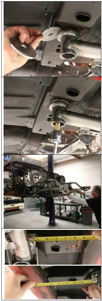
If a torque arm crossmember is not being used, place the spacer up against the floorboard between it and the mounting pad on the front clip, this will allow the proper height.
