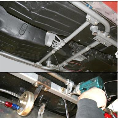
The Torque Arm cross-member is installed with the driveshaft loop facing rearward and the end flanges of the cross-member under the brackets on the subframe connectors. Using the  $3/8 \times 16 \times 1$  inch bolts and washers, bolt the cross-member to the sub-frame brackets and install the 3/8 Nylock nuts and washers. Double check to make sure that the driveshaft loop is centered in the driveshaft tunnel before final tightening.
