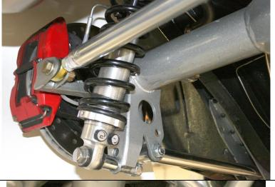
Install the panhard bar to the axle housing bracket using  $\frac{1}{2}$  x 20 x 2 inch bolt, washers and Nylock nut.
