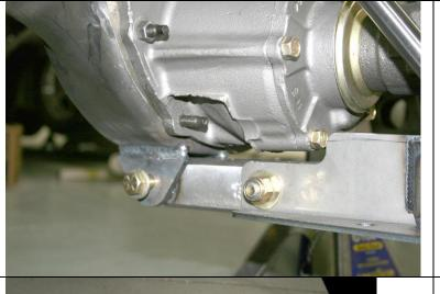
Install the rear of the Torque Arm to the tabs on the bottom of the rear end housing using a  $\frac{1}{2}$  inch by  $\frac{3}{2}$  inch bolt, washers and nut. Lightly tighten.
