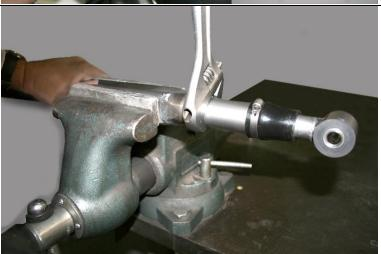
The Torque Arm is shipped with the slider assembly separate to facilitate packaging. The slider has preassembled with Teflon bushings and has been installed in the Torque Arm to check for proper fit. We use anti-seize on the threads to prevent galling. When painting or powder coating the assembly, tape the threads on the slider and plug the hole in the Torque Arm tube.
