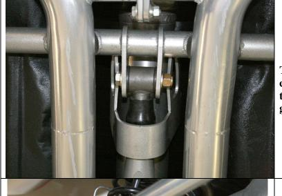
The slider is installed and centered. The Torque Arm cross-member has exhaust cut out relief's to allow the exhaust pipes to be tucked up higher for more ground clearance.
