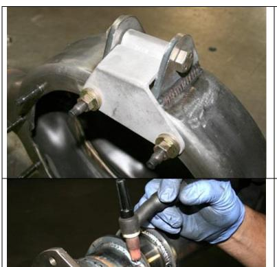
The torque arm tabs are welded on by using the supplied fixture tool. Bolt fixture to the lowest 2 third member bolts flat against the housing flange. Bolt on the two supplied tabs using the  $\frac{1}{2}$  by  $3\frac{1}{2}$  inch bolt and with the longer tab to the passenger side of the housing. Bottom of tabs may need sanding to fit. Weld outside and wrap welds also to the inside.
