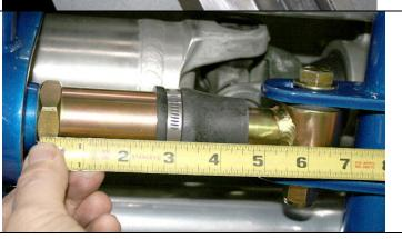
The slider shaft travels in and out very little but still needs to be positioned in the slots 6½ inches from the back of the wrench flats on the housing to the center of the sleeve with the bushing in it. This adjustment allows the slider shaft to be in the middle of its travel. Tighten the Nylock nut.
