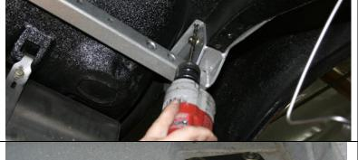
Using the 5/16 inch holes on the flange of the channel bracket as a guide, use a long shank 5/16 drill bit and drill the 4 holes (2 on 68-69) through the floor of the trunk.
