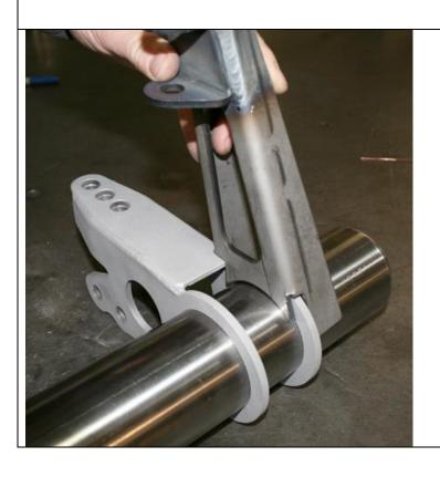
The axle brackets are designed to slide over a 3 inch axle tube before the bearing flange housings are installed. If the bearing ends are already on the axle bracket 3 inch ribs can be cut 90 degrees to the flat shock mounting face and re-attached after the bracket is tacked on. The brackets are positioned 44 1/8 centers for stock width and 40 1/8 for the 2 inch mini-tub.
