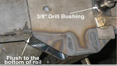
Using a 3/8 inch drill bit and using the 3/8 inch holes in the channel bracket, drill the inside holes through the frame rail. Then using the furnished drill guide, align the drill bit in the guide with the drill bit in the previously drilled hole and clamp the guide as pictured. This will facilitate in keeping the drill bit in line with the outside holes in the bracket.
