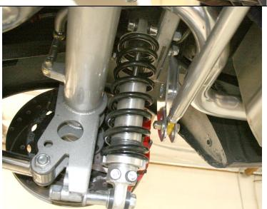
The process is repeated on the right side on the panhard bar bracket that is bolted to the coil-over cross-member. The three hole adjustment gives the choice of raising or lowering the rear roll center. Finish the project by installing the shock hole block off plates using the four 5/16 x 18 x 3/4 button head bolts.
