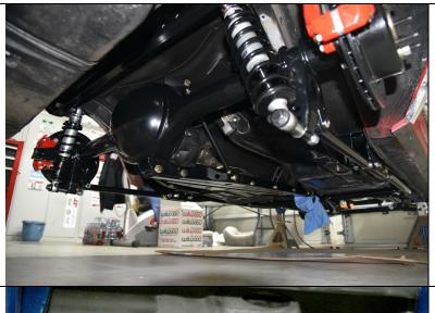
Lift the rear axle into place and connect the link bars. The adjustable side attaches to the chassis.
