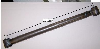
Adjust the link bars to 19.25" center to center. This can be adjusted as needed later.
