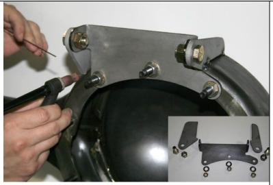
The pinion support brackets are installed next. Using the furnished fixture tool, using the three 3/8 by 24 nuts, bolt the fixture onto the top three studs of the third member housing with the locating tabs facing forward. Bolt the ¼ inch laser cut brackets to the outside of the fixture tool using the two ½ inch bolts with the wider bracket on the passenger side and the shorter bracket on the driver side.
