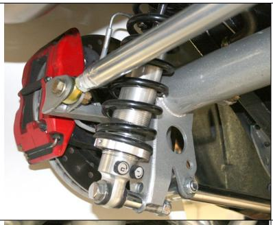
Install the panhard bar to the axle housing bracket using  $\frac{1}{2}$  x 20 x 2 inch bolt, washers and Nylock nut.
