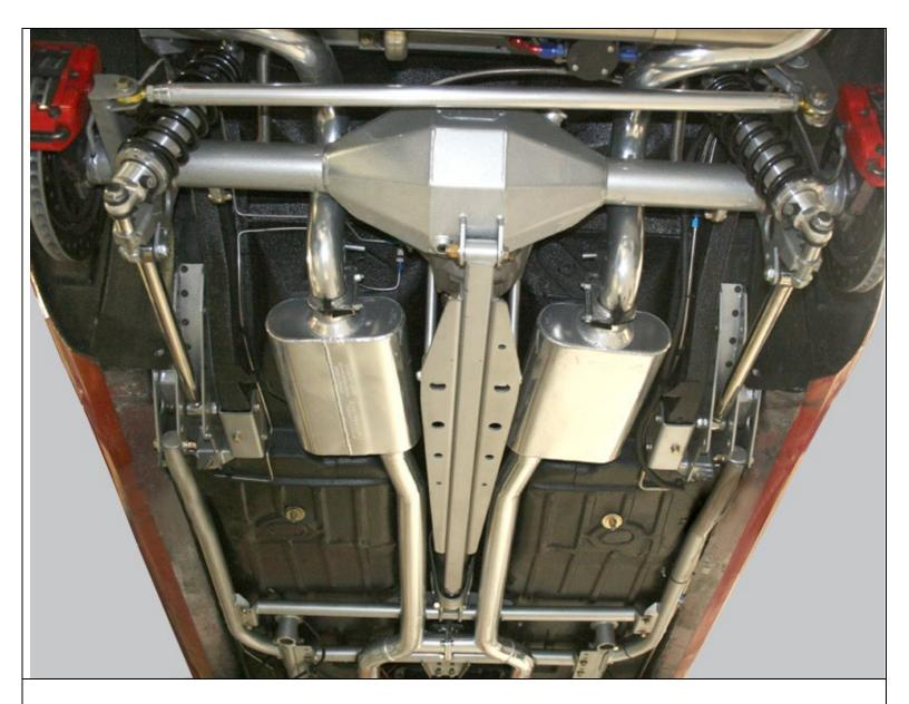
The Torque Arm rear suspension completely installed. Everything is tucked up close and tight so installing the driveshaft should be done before installing exhaust system and leaving one of the pinion support tubes off until the driveshaft is installed.
