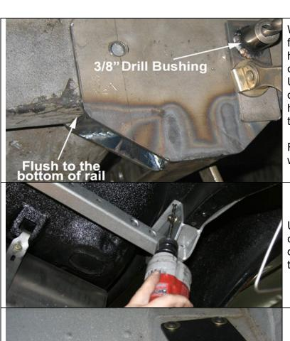
With the channel bracket pressed flush against the frame rail, use a 3/8 drill bit and drill the two outside holes in each frame rail using the holes in the channel bracket as a guide.
