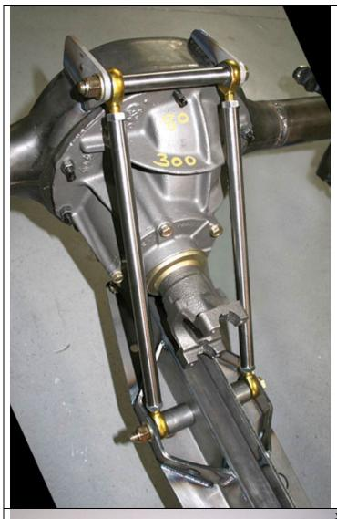
The pinion support tubes have left and right hand rod ends to facilitate pinion angle adjustment. Adjust the tubes to approximately the same length with an equal amount of threads showing on each rod end. Install the tubes with the right hand rod ends on the inside of the top brackets using the ½ by 8 inch bolt, washers, 5.2 inch spacer in between rod ends and Nylock nut.
