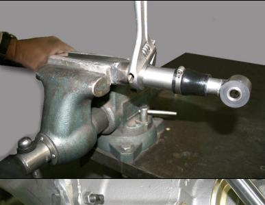
The Torque Arm is shipped with the slider assembly separate to facilitate packaging. The slider has pre-assembled with Teflon bushings and has been installed in the Torque Arm to check for proper fit. We use anti-seize on the threads to prevent galling. When painting or powder coating the assembly, tape the threads on the slider and plug the hole in the Torque Arm tube.
