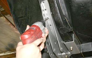
Next using the 5/16 inch bracket holes as a guide, drill one 5/16 hole through the floor pan and install one of the 5/16 x 1½ x 24 button head bolts and install nut on inside and tighten. This will keep the bracket from moving around while drilling and all holes will line up when finished. Finish drilling remainder of the holes using a long shank 5/16 inch drill bit.
