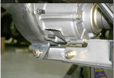
Install the rear of the Torque Arm to the tabs on the bottom of the rear end housing using a ½ inch by 3½ inch bolt, washers and nut. Lightly tighten.
