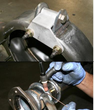
The torque arm tabs are welded on by using the supplied fixture tool. Bolt fixture to the lowest 2 third member bolts flat against the housing flange. Bolt on the two supplied tabs using the ½ by 3½ inch bolt and with the longer tab to the passenger side of the housing. Bottom of tabs may need sanding to fit. Weld outside and wrap welds also to the inside.
