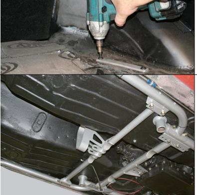
The Torque Arm cross-member is installed with the driveshaft loop facing rearward and the end flanges of the cross-member under the brackets on the sub-frame connectors. Using the 3/8 x 16 x 1 inch bolts and washers, bolt the cross-member to the sub-frame brackets and install the 3/8 Nylock nuts and washers. Double check to make sure that the driveshaft loop is centered in the driveshaft tunnel before final tightening.
