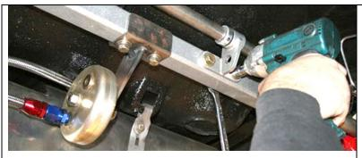
When installing the optional ¾ inch rear sway bar, first slide the lock rings on. Next the split urethane bushing with flange facing lock ring. Next the brackets with the flange facing rearward and the sway bar forward. Leave lock rings loose to facilitate install. Install the four 3/8 x 2½ bolts, washers and Nylock nuts. Adjust sway bar location after rear axle is installed. Note: We mounted the fuel filter and pump to the cross-member.
