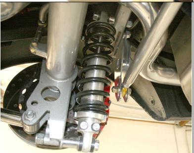
The process is repeated on the right side on the panhard bar bracket that is bolted to the coil-over cross-member. The three hole adjustment gives the choice of raising or lowering the rear roll center. Finish the project by installing the shock hole block off plates using the four 5/16 x 18 x ¾ button head bolts.
