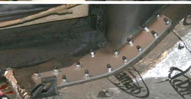
Align the appropriate curved re-enforcing plate on the inside of the car over the drilled bolt holes and have a second person push the 5/16 button headed bolts through the bracket underneath. Install the washers and the 5/16 Nylock nuts and tighten.
