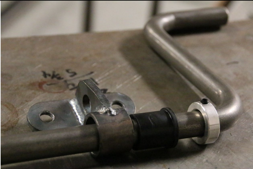
Optional anti-sway bar installation: See the photo on the left for assembly of the sway bar mounting flange, bushing and retainer.
