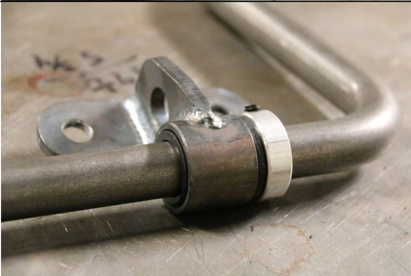
Apply urethane energy grease to the inside of the bushing and slide it into the mounting flange. Leave the retaining collar loose for now. Use the provided 3/8" heims and hardware to install the arms onto the special shoulder bolts at the top 4-link bar attachment.
