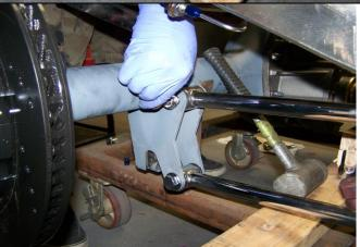
Place the upper 4-link bar onto the upper hole of the axle bracket using the provided 5/8" hardware.
