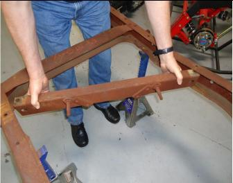
Remove the factory shock cross member using the same process as before with the leaf spring brackets.
