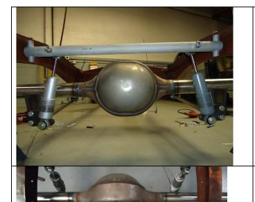
You can now install the coil-overs using the provided 5/8" hardware and spacers. The threaded side of the shock goes down as per the picture.
