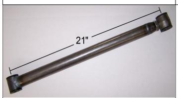
Adjust all the 4-link bars to 21" center to center and tighten the leave the jam nuts finger tight.
