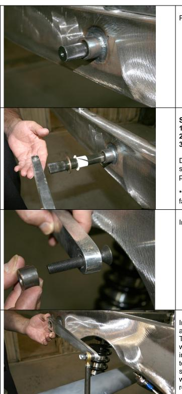
Place the splined bar into the housing.
