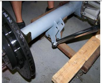
Move the rear axle into place underneath the frame near wheel centerline.
