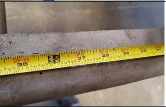
Measure from the center of the rear bed hole going forward. Make a mark at 29.5" on both passenger and driver side frame rails.
