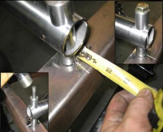
Set the cross member on top of the rails at 29.5" centers. Center the cross member fore and aft on the line. Take measurements on both passenger and driver side in order to center the cross member from side to side as pictured.
