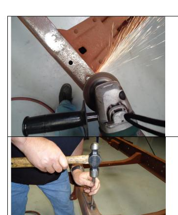
This picture was taken with the frame flipped upside down to get a better shot. The two rivets holding the stock cross member must be removed in order to install the 4-link frame brackets.
