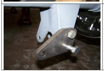
Install the offset axle brackets onto the axle brackets using the provided 5/8" hardware. These are designed to keep the coil-overs from making contact with the frame rail as the suspension compresses. The flat area of the plate will sit parallel to the ground and the shock hole will sit inboard of the bracket when properly installed.
