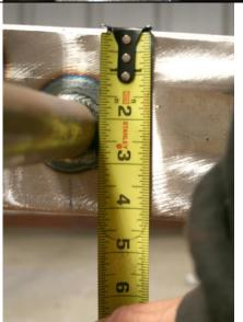
Measure down 2 1/8" down from the top of the rail at the mark you just made. Use a center punch to mark the frame where these two measurements intersect. This is the anti-roll bar housing centerline.
