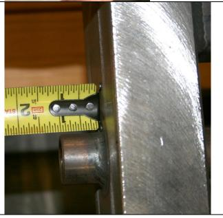
Place the housing through the frame making sure it protrudes the same distance on both sides.
