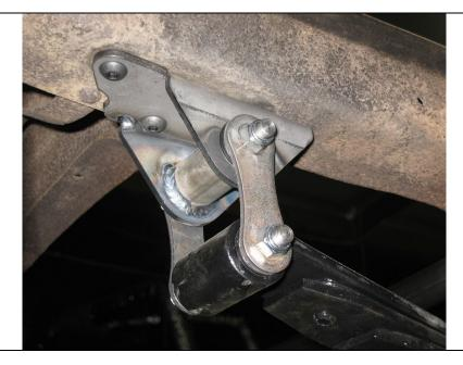
The bolt for the bracket hole under the welded tube will have to be inserted from inside the frame railed with the nut inside the bracket. The nut is under the tube and is not visible in this picture.
