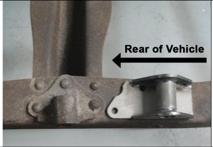
Remove the stock rear shackle bracket rivets in the same manner as the front spring hanger bracket rivets. The shackle brackets are positioned on the rails with the welded side on the inside of the rail. Line up the brackets with the holes of the original brackets. It may be necessary to align-drill a couple of these holes. Use three 3/8-16 x 1" bolts, nuts, and one washer under each nut to fasten each bracket. The square front edge of the bracket faces to the front of the vehicle.
