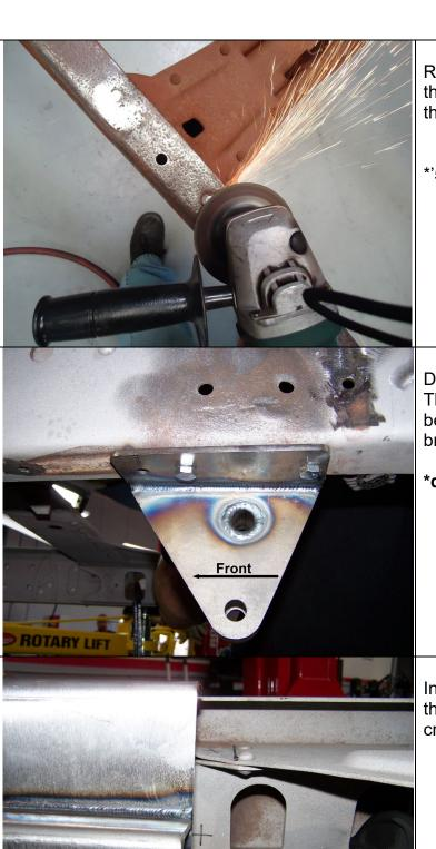
Remove the front leaf spring mounts by grinding off the rivet heads and then punch the rivets body through the frame.
