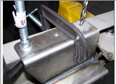
Once the brackets are in the proper position use a couple c-clamps to hold them in place. Tighten down the existing bolts to help keep the brackets in place.
