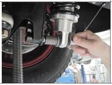
You can now install the coil-overs using the provided 5/8" hardware. The threaded side goes down as per the picture.
