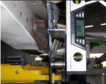
We need to make sure the brackets are square to each other and are sitting vertical before drilling any holes.
