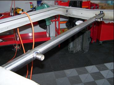
Place the new coil-over cross member into the frame rail with the extended tube for the shock mount pointing forward.
