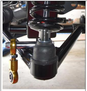
Next, install the shock into the lower a-arm tabs making sure that the adjustment dial faces towards the ball joint and install the 3 ¾ inch shoulder bolt from the rear through the rear tab, then the shock bearing, front tab, then the spacer and last the rod end link for the sway bar. Install the washer and nut and tighten. The top rod end will be attached to the sway bar later.
