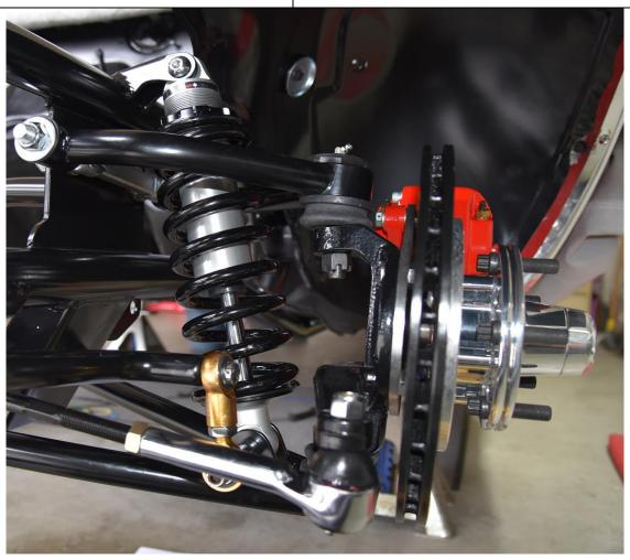
The spindle assembly is installed next. Align the ball joint shafts so the cotter pins can be installed from front to rear. This will help later. Set the spindle assembly on the lower ball joint with the steering arm facing forward and the brake caliper towards the rear. Install the washer & castle nut. Pull the upper a-arm ball joint down into the top of the spindle and install the washer & nut. nut, tighten both castle nuts and install cotter pins. Bend the pins to retain the nuts.
