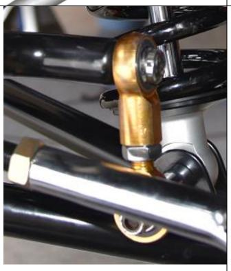
Complete installation by fastening the upper  $\frac{1}{2}$  inch rod end of the sway bar link from the lower shock mount bolt to the end of the anti-roll bar with the  $\frac{1}{2}$ -20 x 1  $\frac{1}{2}$  inch button head bolt.
