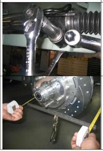
Install the rack & pinion assembly using the two 5/8" in. bolts, washers and lock nuts supplied. On power rack and pinions units the 5/8 thick spacer goes between the rack brackets on the cross member and the rack. Install the tie rod ends onto the rack and into the spindle steering arms.
