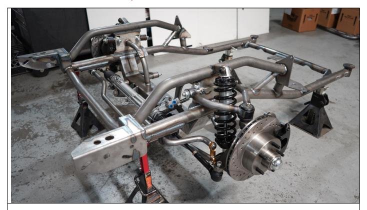
Thank you for choosing TCI Engineering's Chevy Camaro/Firebird/Nova front suspension package. The kit has been designed to not only allow your car to handle corners, steer, brake better and have more engine compartment room but have that low pro touring stance.
