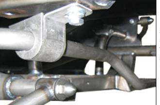
Install the front anti-roll bar into position using the supplied polyurethane and saddle mount making sure that the stepped down center section is down to clear the engine pulley. Fasten anti-roll bar saddle mount using the supplied 3/8-16 x 1 inch hex head bolt; 3/8 inch lock and flat washer.
