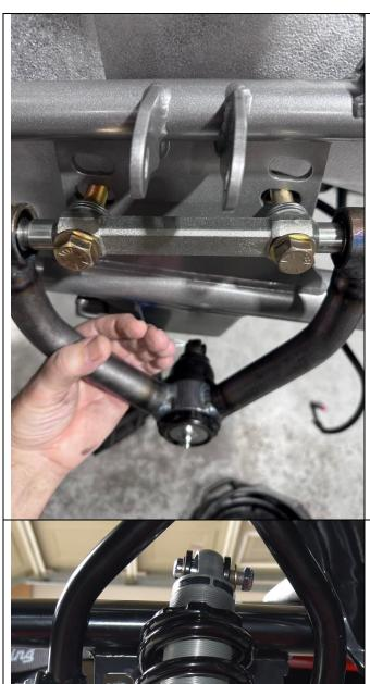
Install the upper control arm into position.
