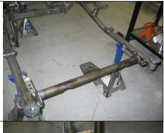
The TCI Camaro/Firebird/Nova clip comes with an adjustable transmission cross-member to accommodate different types of Chevy transmissions. Fasten with the supplied 3/8-16 x 1½ inch Gr. 8 Hex Head Bolt and 3/8 inch full height Nyloc nut.
