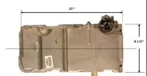
If you are running an LS series engine you must use the F-Body oil pan listed below to have the proper clearance between the rack and the oil pan.
