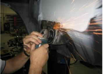
Prep the firewall mounting surface edge on the firewall side by grinding smooth the flange edge so that the TCI clip will be mounted flush to the firewall.
