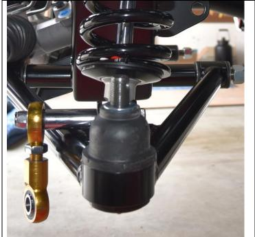
Next, install the shock into the lower a-arm tabs. The rebound adjuster can face either, we recommend inward. Install the 3 ¾ inch shoulder bolt from the rear through the rear tab, then the shock bearing, front tab, then the spacer and last the rod end link for the sway bar. Install the washer and nut and tighten. The top rod end will be attached to the sway bar later.
