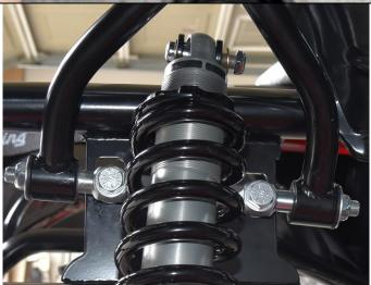
Install the shock to the upper mount using the supplied  $\frac{1}{2}$  -20 by 1  $\frac{3}{4}$  inch button head bolt and  $\frac{1}{2}$  -20 half height nut.
