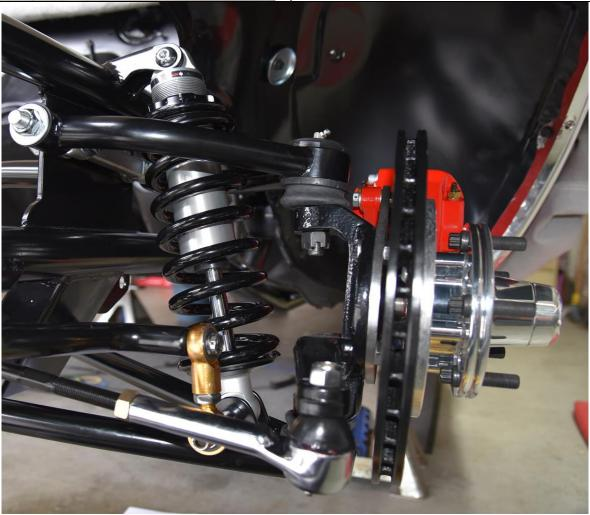
The spindle assembly is installed next. Align the ball joint shafts so the cotter pins can be installed from front to rear. This will help later. Set the spindle assembly on the lower ball joint with the steering arm facing forward and the brake caliper towards the rear. Install the washer & castle nut. Pull the upper a-arm ball joint down into the top of the spindle and install the washer & nut. nut, tighten both castle nuts and install cotter pins. Bend the pins to retain the nuts.
