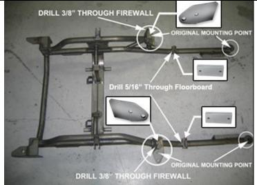
Start the installation of the new sub-frame by raising it up into the original mounting position. A floor-jack will be helpful here. Line up the holes in the firewall and the far rear mounting points and fasten it using the new supplied bolts, lock washer and flat washer (Qty. 4 5/8-11 x 2" Gr. 8 Hex Head) Using a 15/16" shallow socket. Do not tighten up the bolts at this time until all mounting bolts have been started then tighten and secure to the body.
