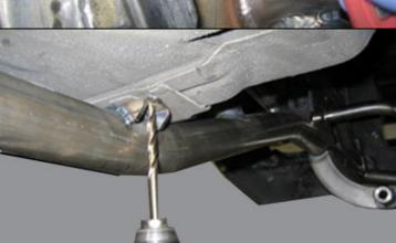
Next, drill 2 holes (per side) through the floorboard located between the firewall mounting point and the rear-most mounting point using a 5/16" drill bit.
