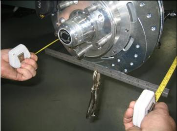
Clamp a straight edge to each rotor as shown then using a tape measure front and rear; set the toe-in approximately 1/8" for a starting point.
