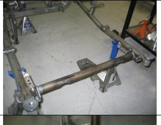
The TCI Camaro/Firebird/Novclip comes with an adjustable transmission cross-member to accommodate different types of Chevy transmissions. Fasten with the supplied 3/8-16 x 1½ inch Gr. 8 Hex Head Bolt and 3/8 inch full height Nyloc nut.
