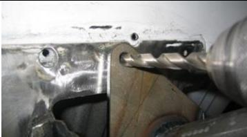
Drill 3/8 holes through the firewall using the mounting bracket as a guide.
