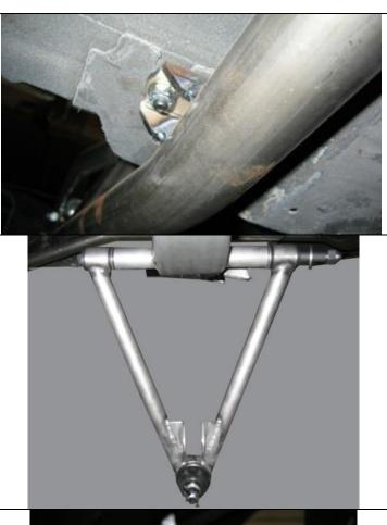
Fasten by using a 5/16" Button Head Bolts with the head of the bolt inside the car.
