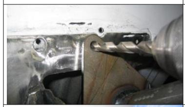
Drill 3/8 holes through the firewall using the mounting bracket as a guide.
