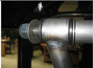
After inserting the control arm bolt from the front to the rear, place the supplied flat washers between each side of the polyurethane bushing. Complete assembly by tightening the 5/8" full Nyloc nut.
