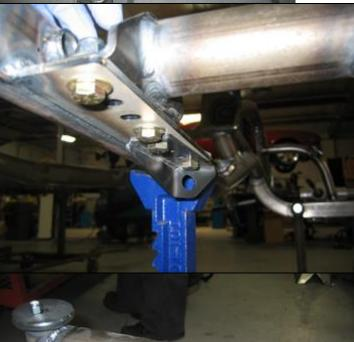
Mount the emergency brake cable bracket on the driver side with the same mounting point as the transmission cross-member.
