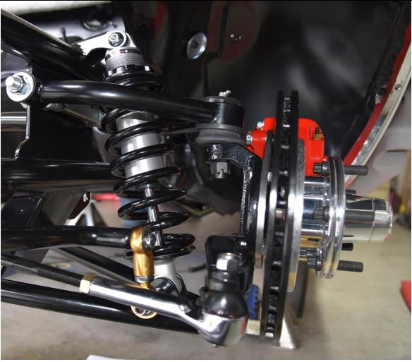
The spindle assembly is installed next. Align the ball joint shafts so the cotter pins can be installed from front to rear. This will help later. Set the spindle assembly on the lower ball joint with the steering arm facing forward and the brake caliper towards the rear. Install the washer & castle nut. Pull the upper arm ball joint down into the top of the spindle and install the washer & nut. nut, tighten both castle nuts and install cotter pins. Bend the pins to retain the nuts.
