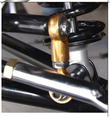
Complete installation by fastening the upper  $\frac{1}{2}$  inch rod end of the sway bar link from the lower shock mount bolt to the end of the anti-roll bar with the  $\frac{1}{2}$ -20 x 1  $\frac{1}{2}$  inch button head bolt.
