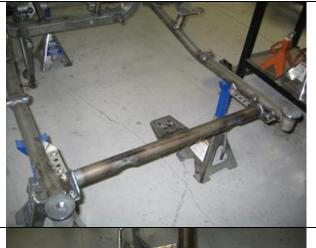
The TCI Camaro/Firebird/Nova clip comes with an adjustable transmission cross-member to accommodate different types of Chevy transmissions. Fasten with the supplied 3/8-16 x 1½ inch Gr. 8 Hex Head Bolt and 3/8 inch full height Nyloc nut.
