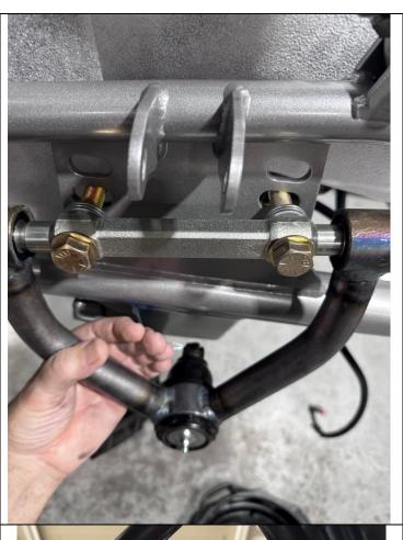
Install the upper control arm into position.
