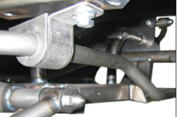
Install the front anti-roll bar into position using the supplied polyurethane and saddle mount making sure that the stepped down center section is down to clear the engine pulley. Fasten anti-roll bar saddle mount using the supplied 3/8-16 x 1 inch hex head bolt; 3/8 inch lock and flat washer.
