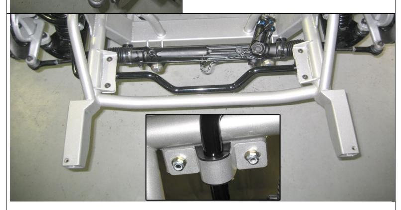
21. Installing the Anti-Sway Bar.
