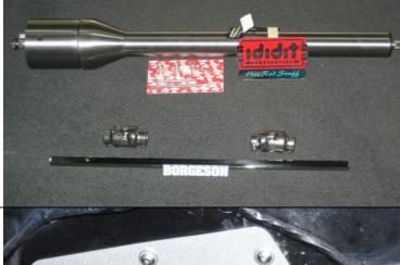
The stock steering column can be cut and modified to work but I chose an Ididit brushed steel two inch diameter tilt retro fit steering column (TCI # 326-3100-00) and a Borgenson steering linkage package (TCI # 310-3120-03) to connect the rack and pinion to the steering wheel.
