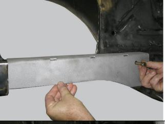
You are now ready to start installing the boxing plates to strengthen the frame in the cross member area.
