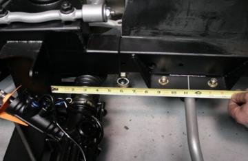
The sway bar bracket is mounted 11.25 inches from the front edge of the cross member to the center of the bracket.
