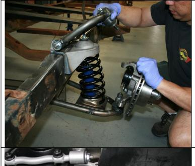
Pull the upper control arm down onto the spindle. Place the ball joint washer first and then the castle nut. Torque the upper ball joint to 70 ft. lbs and install the cotter pin. The upper ball joint is a **MOOG K772**
