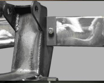
You are now ready to install the cross member. First install the one inch wide locating plate using a 3/8" bolt through the hole drilled earlier. Slide the cross member with the rack & pinion brackets up against the locating plate.
