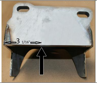
The control arm shock/coil spring tower bracket is mounted with the tall end towards the front of the car. This is the built in anti-dive feature. Set the control arm shock/coil spring tower in place with the front face 3 1/16" from the front face of the cross member.
