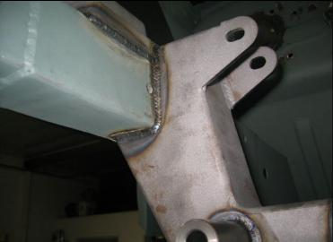
Double check for square and tack weld all sides and on the bottom.
