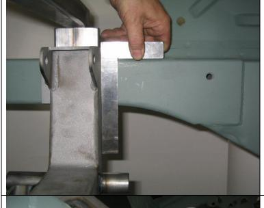
Check to make sure that the cross member is 90 degrees to the top of the frame. This is critical for correct engine angle and lower A-arm angle.
