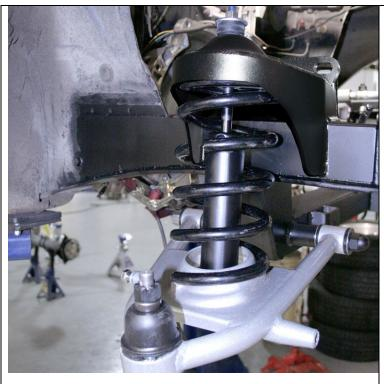
We suggest that you wait until final vehicle assembly (vehicle at full weight) to install the coil springs because it will put undue stress on the ball joints and could cause the boots to tear. Another option is to remove the upper and lower ball joint boots and then cover the ball joints to keep dirt out until you're ready to drive the vehicle.
