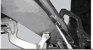
The outside edge of the frame is where the two stamped flanges of the frame are spot welded together and will require clearance grinding for the coil spring before welding.
