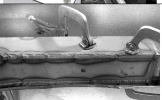
Using the outer edge of the lower boxing plate as the template, grind the two stock frame flanges till they match the profile of the boxing plate edge.
