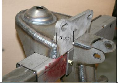
Using a C-clamp pull the bracket down snug to the top of the frame rail keeping the locating slot aligned with the front edge of the cross member and the outside legs of the bracket snug against the outside of frame rail. The mounting plate for the upper control arm should be vertical +/- .5 degrees.
