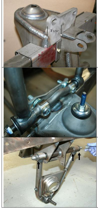
Using a C-clamp pull the bracket down snug to the top of the frame rail keeping the locating slot aligned with the front edge of the cross member and the outside legs of the bracket snug against the outside of frame rail. The mounting plate for the upper control arm should be vertical +/- .5 degrees.
