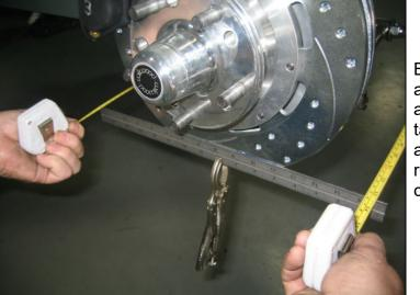
Before installing the tie rod ends onto the rack assembly, align the rotors straight forward and clamp a straight edge to each rotor as shown then using a tape measure side to side; set the toe-in approximately 1/8" for a starting point. Adjust the tie rods onto the rack assembly evenly to keep the rack centered for equal turning left and right.
