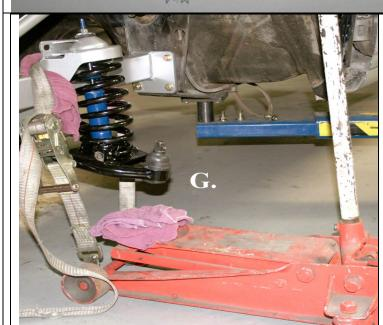
5. **(Image F)** Install the shock through the bottom of the lower a-arm with the shock stem going through the mounting hole in the upper hat. Align the lower shock sleeve with the shock bosses on the lower a-arm and install the 7/16" shock bolt and tighten
