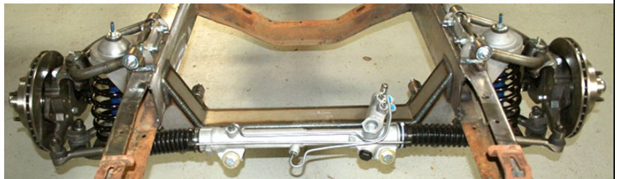
New Coil-Spring Front End on a Stock Chassis
