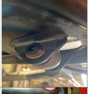
Extend the shock through the cutout in the lower aarm and install the bolt, washers and ½ Nylock nut. Tighten securely.
