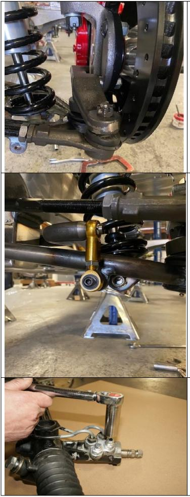
Install the jam nut and outer tie rod end onto both sides of the rack. With the rotors pointing straight ahead (0 toe) install the tie rod ends into the bottom of the steering arm. Torque the tie rod ends to 60 ft. lbs. and install the cotter pin.
