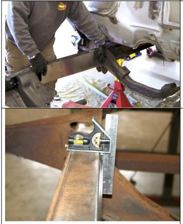
It is important that the boxing plates be positioned on the edge of the frame rail so that you can maximize weld penetration. This will insure there is enough weld to grind and smooth out the corners.
