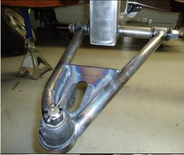
The 4<sup>th</sup> and final washer can now be placed on the 5/8" shaft and the Nylock can be installed.
