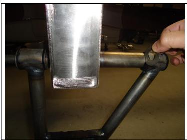
Place the 3rd washer in between the bushing and the pin as shown.
