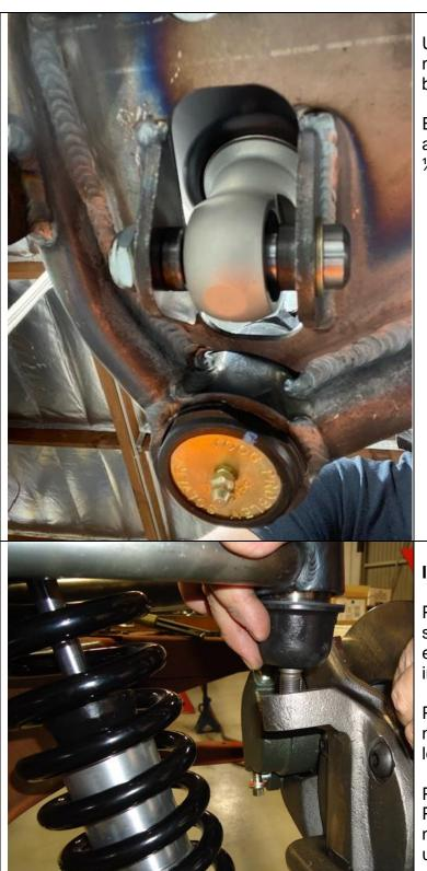
Use **BOLT\_KIT\_002\_P/U**, the bottom bolt has a modified head that needs to be installed from the back to the front.
