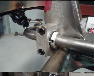
The anti-sway bar mounts to the rear of the cross member above the lower control arm pins. Use the supplied hardware to install the aluminum blocks onto the cross member. Torque to 30 ft lbs.
