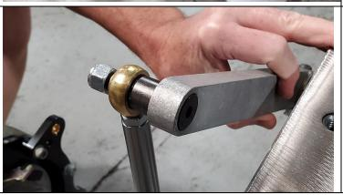
Using **SWY\_BAR\_HIEMS38+3-P**, assemble the sway bar links.
