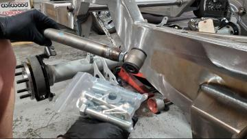
Using **Bolt Kit 108**, install the 2-link bars with the adjuster side onto the frame using the provided 5/8" hardware. The bolts go in from the outside of the frame which will place the nylock on the inboard side.
