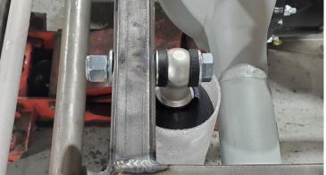
Also using **Bolt Kit 061**, install the top & bottom of the shock as shown.
