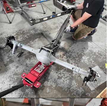
Place the rear end assembly with the torque arm onto a floor jack and roll it under the chassis.
