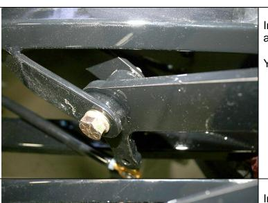
Install the provided hardware into the frame mount and through the pivot pin of the pedal arm.
