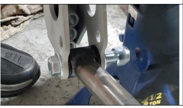
Align the axle assembly under the chassis and install the rear of the link bars.
