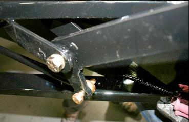
Install the left-handed hiem and jam nut into the pushrod and install the assembly on the outboard side of the pedal arm.
