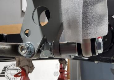
Install the bottom of the shock with spacer as shown.
