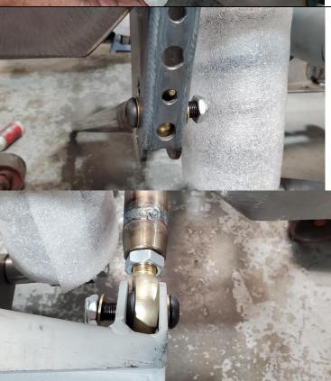
Install bar into the chassis bracket and the opposite side into the rear end housing.
