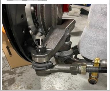
Install the jam nut and outer tie rod end onto both sides of the rack. With the rotors pointing straight ahead (0 toe) install the tie rod ends into the bottom of the steering arm. Tighten the castle nut and install the cotter pin.
