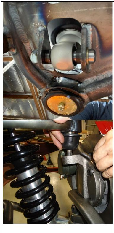
The bottom bolt has a modified head that needs to be installed from the front to the back.
