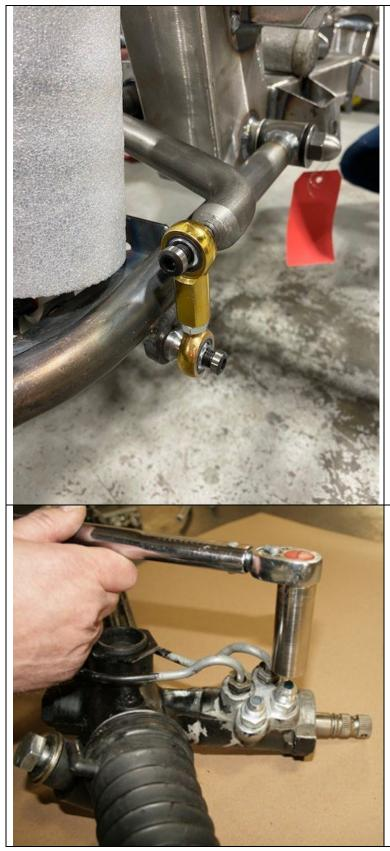
The sway bar routes from behind the cross member above the lower control arms and hooks up to the front of the control arms. Use the supplied hardware to install the rod ends with the male on the bottom.
