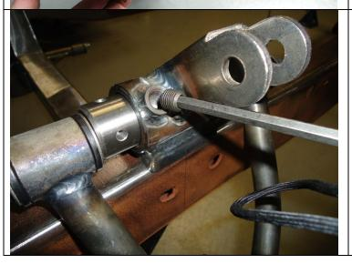
Install the  $\frac{1}{2}$ -20 set screws into the Eccentric housing and tighten.
