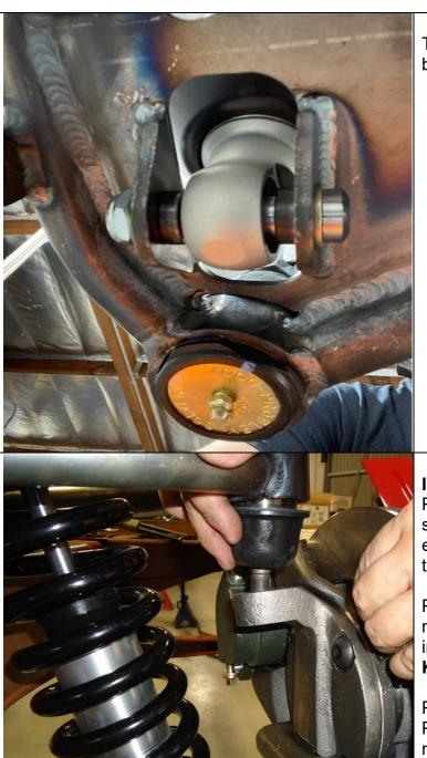
The bottom bolt has a modified head that needs to be installed from the front to the back.
