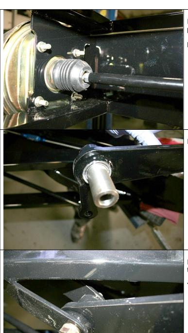
Installing the Pedal assembly: Thread the R/H end of the provided rod into the back side of the booster.
