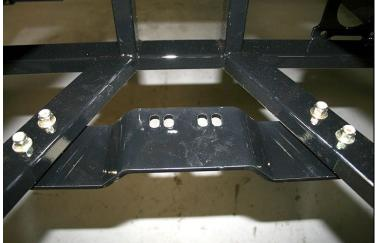
Install the transmission mount as shown. Your crossmember may sit closer or farther away from the chassis cross bar depending on which transmission you are using.
