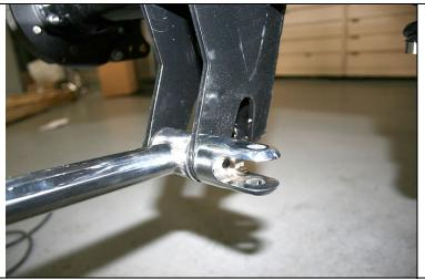
**\*NOTE\*** The passenger side rear lower link bar does not use a nylock nut, rather a clevis for attaching the track bar. Install the clevis onto this bolt at this time.
