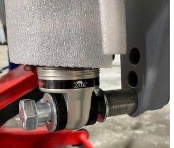
The coil-over mount will have a spacer. Use a washer up against the spacer and the bolt head.
