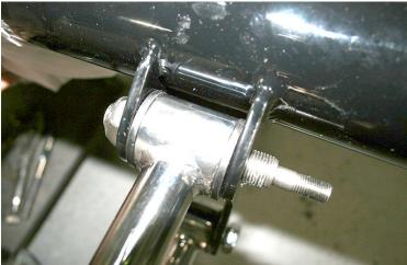
Install one rod end of the track bar onto either clevis and use it as leverage to tighten it down(125 ft lbs). Remove the rod end from that clevis and repeat this process on the other clevis.
