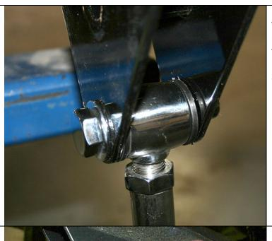
\*NOTE\* The driver's side front lower link bar does not use a nylock nut, rather a clevis for attaching the track bar.
