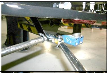
You may need to rotate the clevis so that the 9/16" bolts holding the rod end are sitting vertical. Install the track bar completely onto the clevises. Make sure the rear end is centered in the frame and that the wheel base is correct by adjusting the Link & Track bars accordingly. Tighten down the jam nuts on the Track and 4-link bars.
