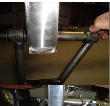
Place the 3rd washer in between the bushing and the pin as shown.
