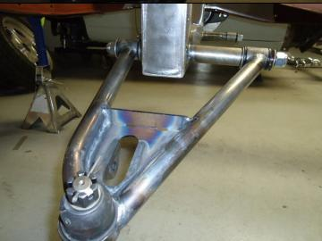
The 4<sup>th</sup> and final washer can now be placed on the 5/8" shaft and the Nylock can be installed.
