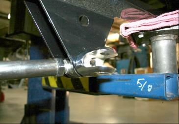
Install the clevis onto this bolt at this time.
