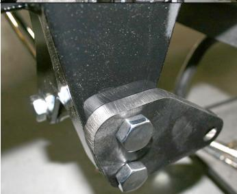
Install the offset axle brackets onto the axle brackets using the provided 5/8" hardware. These are designed to keep the coil-overs from making contact with the frame rail as the suspension compresses.
