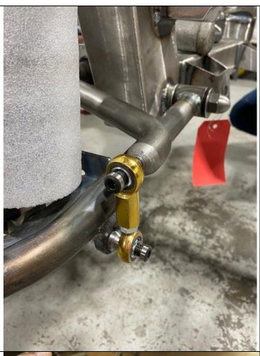
The sway bar routes from behind the cross member above the lower control arms and hooks up to the front of the control arms. Use the supplied hardware to install the rod ends with the male on the bottom.
