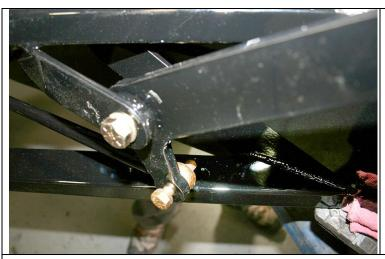
Install the hardware with the heim joint on the outboard side of the pedal arm.
