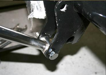
Place the lower 4-link bars onto the lower hole of the axle bracket using the provided 5/8" hardware.
