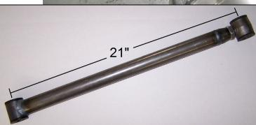
Adjust all the 4-link bars to 21" center to center and tighten the jam nuts.
