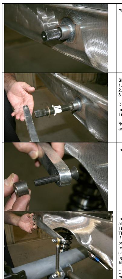
Place the splined bar into the housing.
