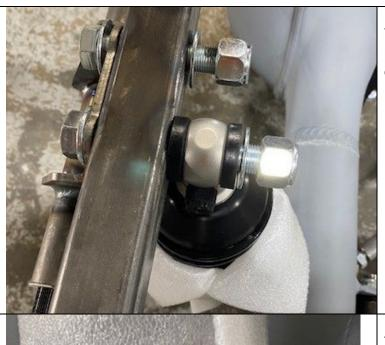
You can now install the coil-overs using the provided 5/8" hardware. The threaded side goes down as per the picture.
