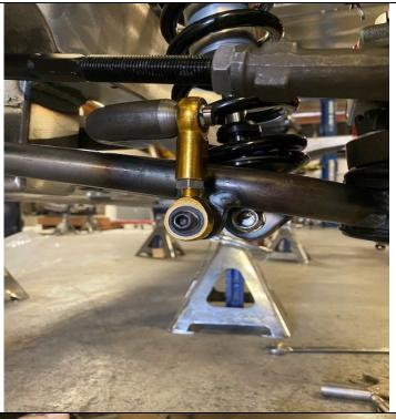
The sway bar routes from behind the cross member above the lower control arms and hooks up to the front of the control arms. Use the supplied hardware to install the rod ends with the male on the bottom.
