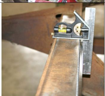
Use a square to make sure that the plates are square to the frame. Tack weld all 4 corners of the plate to the rail and make sure they are still square. Once the boxing plates are confirmed square you can begin welding them in place. Weld 6" sections at a time switching from driver to passenger so heat is kept to a minimum.
