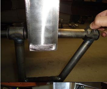
Place the 3rd washer in between the bushing and the pin as shown.
