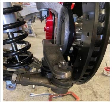
Install the jam nut and outer tie rod end onto both sides of the rack. With the rotors pointing straight ahead (0 toe) install the tie rod ends into the bottom of the steering arm. Torque the tie rod ends to 60 ft. lbs. and install the cotter pin.
