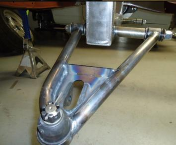
The 4<sup>th</sup> and final washer can now be placed on the 5/8" shaft and the Nylock can be installed.
