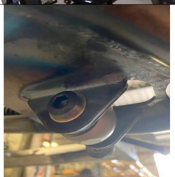
The bottom bolt is longer and has a modified head that needs to be installed from the back to the front.
