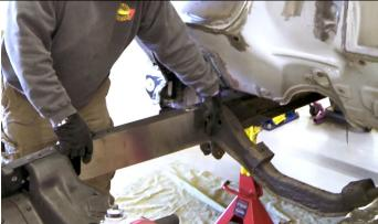
It is important that the boxing plates be positioned on the edge of the frame rail so that you can maximize weld penetration. This will insure there is enough weld to grind and smooth out the corners.
