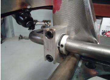
The anti-sway bar mounts to the rear of the cross member above the lower control arm pins. Use the supplied hardware to install the aluminum blocks onto the cross member. Torque to 35 ft lbs.
