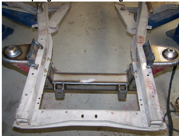
New Coil-Spring Front End on Original Stock Chassis
