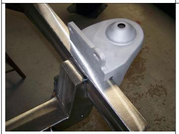
Once proper placement is confirmed a couple tack welds can be placed at the top and side of the tower/frame.
