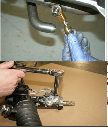
The sway bar routes from behind the cross member under the control arms and hooks up to the front of the control arms. Use the supplied hardware to install the heim joints with the male on the bottom.
