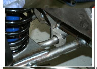
The anti-sway bar mounts to the rear of the cross member below the lower control arm pins. Use the supplied hardware to install the aluminum blocks onto the cross member. Torque to 35 ft lbs.
