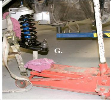
5. **(Image F)** Install the shock through the bottom of the lower a-arm with the shock stem going through the mounting hole in the upper hat. Align the lower shock sleeve with the shock bosses on the lower a-arm and install the 7/16" shock bolt and tighten
