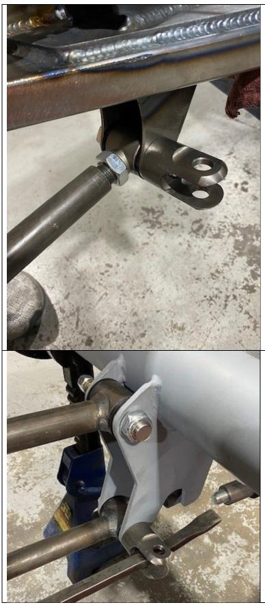
**\*NOTE\*** The driver's side front lower link bar does not use a nylock nut, rather a clevis for attaching the track bar. The clevis is on the track bar assembly for shipping. See picture below.
