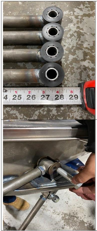
Adjust all the 4-link bars to 27.5" center to center and tighten the jam nuts.
