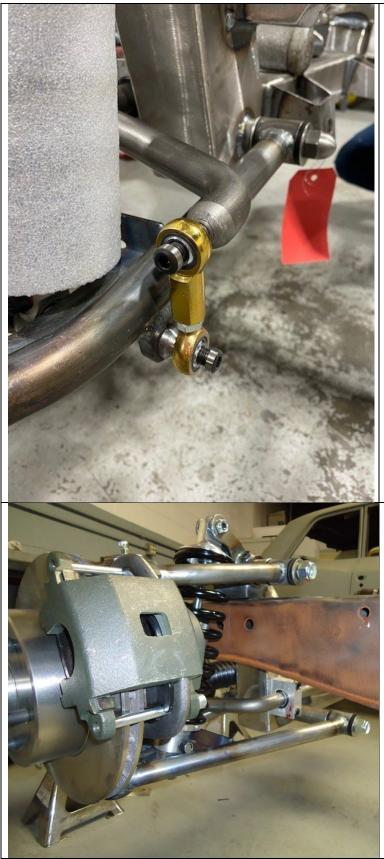
The sway bar routes from behind the cross member above the lower control arms and hooks up to the front of the control arms. Use the supplied hardware to install the rod ends with the male on the bottom. Note the spacer used between the hiem joint and A arm tab.
