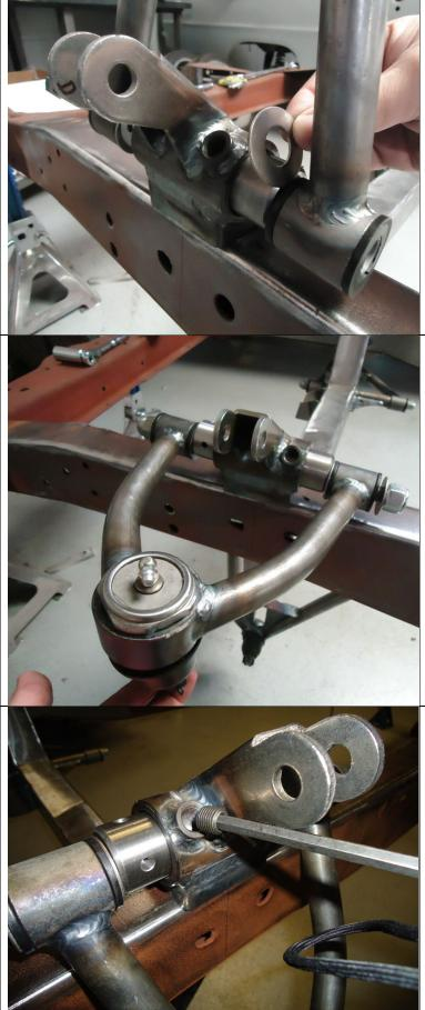
Place the 3rd washer in between the bushing and the eccentric as shown.
