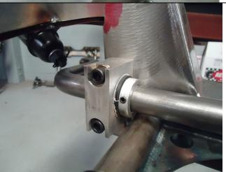
The anti-sway bar mounts to the rear of the cross member above the lower control arm pins. Use the supplied hardware to install the aluminum blocks onto the cross member. Torque to 25 ft lbs.
