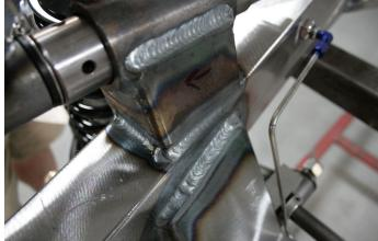
Double check all measurements and finish welding the cross member and eccentric housings into place.
