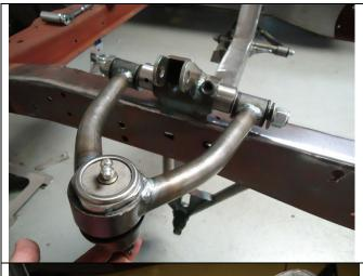
The 4<sup>th</sup> and final washer can now be placed on the 5/8" shaft and the Nylock can be installed.
