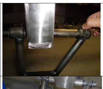
Place the 3rd washer in between the bushing and the pin as shown.
