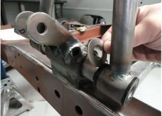
Place the 3rd washer in between the bushing and the eccentric as shown.
