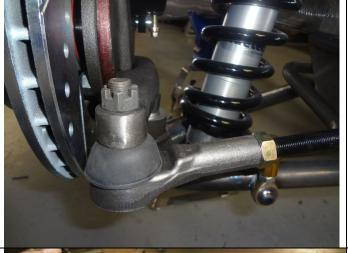
Install the jam nut and outer tie rod end onto both sides of the rack. With the rotors pointing straight ahead (0 toe) install the tie rod ends into the bottom of the steering arm. Torque the tie rod ends to 60 ft. lbs. and install the cotter pin.
