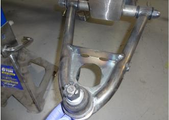
The 4<sup>th</sup> and final washer can now be placed on the 5/8" shaft and the Nylock can be installed.
