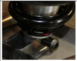
Place the shock onto the lower control arm and install the provided ½" button head bolt.
