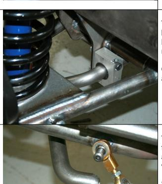
The anti-sway bar mounts to the rear of the cross member below the lower control arm pins. Use the supplied hardware to install the aluminum blocks onto the cross member. Torque to 35 ft lbs.
