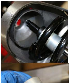
You can now lift the lower control arm and shock/spring combo up into the upper hat assembly. Align the shock shaft into the center hole of the upper hat.
