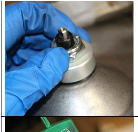
Reinstall the nylock and tighten it down
