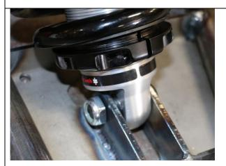
Install the nylock on the opposite side and tighten down
