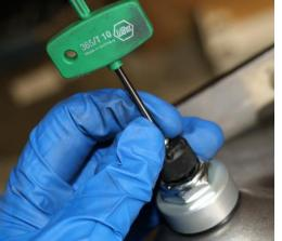
Using the same T10 Torx you can now reinstall the adjuster knob and screw
