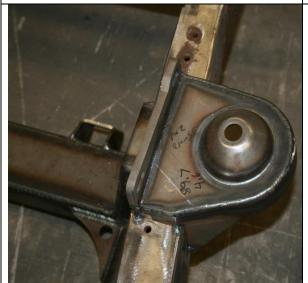
Once proper placement is confirmed a couple tack welds can be placed at the top and the side of the tower/frame.
