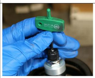
Use a T10 Torx head to remove the screw at the top of the shock/adjuster knob.
