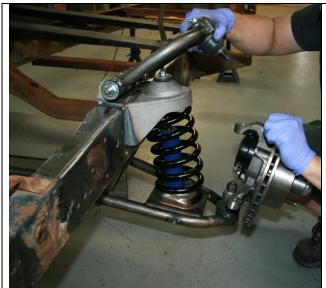
Pull the upper control arm down onto the spindle. Place the ball joint washer first and then the castle nut. Torque the upper ball joint to 70 ft. lbs and install the cotter pin. The upper ball joint is a **MOOG K772**
