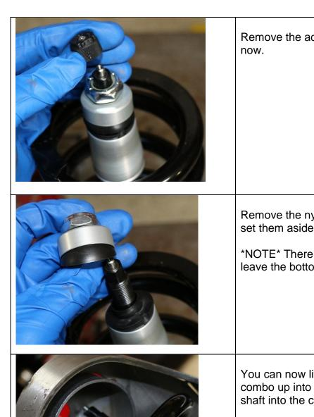
Remove the adjuster knob and screw and set it aside for now.
