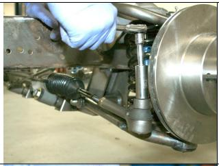
Install the jam nut and outer tie rod end onto both sides of the rack. With the rotors pointing straight ahead (0 toe) install the tie rod ends into the bottom of the steering arm.
