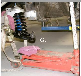
5. (Image F) Install the shock through the bottom of the lower aarm with the shock stem going through the mounting hole in the upper hat. Align the lower shock sleeve with the shock bosses on the lower a-arm and install the 7/16" shock bolt and tighten
