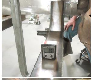
2 degrees frame rake (vehicle stance) is typical. The flat area on top of the cross member should be level to the ground or 0 degrees when the frame is at proper rake.
