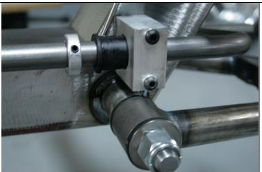
The anti-sway bar mounts to the rear of the cross member above the lower control arm pins. Use the supplied hardware to install the aluminum blocks onto the cross member. Torque to 35 ft lbs.Center the anti-sway bar and lock down the set screws against the bushings.
