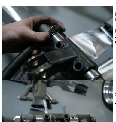
Place the 3rd washer in between the bushing and the eccentric as shown.
