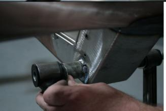
Place the 3rd washer in between the bushing and the pin as shown.
