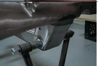
The 4<sup>th</sup> and final washer can now be placed on the 5/8" shaft and the Nylock can be installed.
