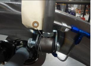
Install the adjuster side of the panhard bar onto the chassis bracket as shown using the provided hardware.
