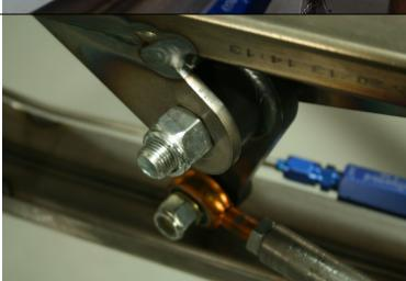
Install the provided hardware into the frame mount and through the pivot pin of the pedal arm. The heim joint goes on the outboard side of the pedal arm.
