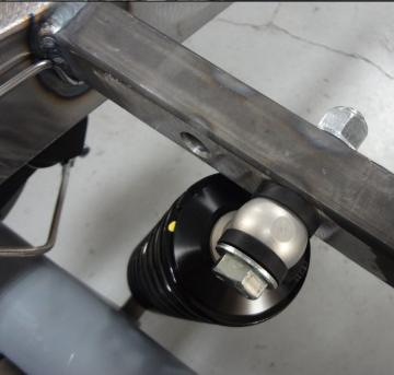
\*NOTE\* Installing the optional Ridetech adjustable shocks.
