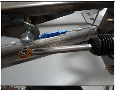
The existing bolt and inner sleeve will have to be removed before installation. Take care when removing the inner sleeve as it is reused on the pedal arm itself.
