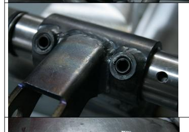
Install the  $\frac{1}{2}$ -20 set screws into the Eccentric housing and tighten.
