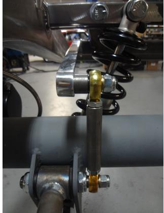
Here is how the finalized installation of the anti-sway bar will look.
