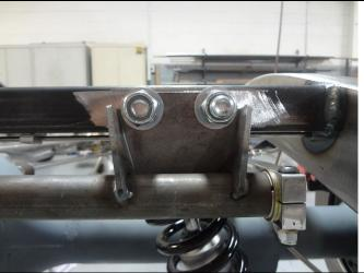
Place the anti-sway bar crossmember up to the back of the coil-over crossmember lining up the two sets of holes on either side of the crossmember
