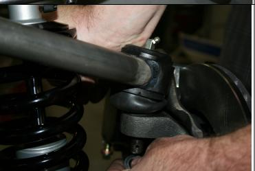
Pull the upper control arm down onto the spindle. Place the ball joint washer first and then the castle nut. Torque the upper ball joint to 70 ft. lbs and install the cotter pin. The upper ball joint is a **MOOG K772**
