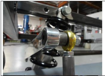
The lower 3/8" rod end connects to the upper 4-link bolt. This is where the special shoulder bolt should be installed. If you haven't installed this bolt already during the 4-link process you will need to remove the upper link bolt and replace it with the provided shoulder bolt. The shoulder side should face inwards. Install the short 5/8" nylock and then tighten it down. The rod end goes on next and the the 3/8" nylock onto the small end of shoulder bolt.
