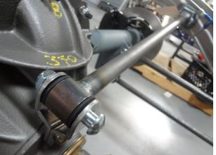
Pull the panhard bar down into place and install the provided hardware.
