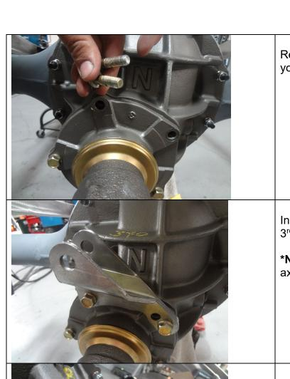
Remove these two bolts from the pinion support on your new 9" axle housing.
