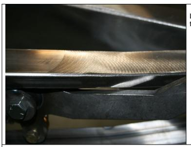
Leave the jam nut loose. Final adjustment will be done once the body is installed and carpet is in place.
