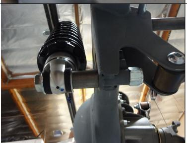
Install the provided spacer up against the back of the axle bracket.
