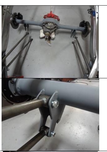
Place the rear axle onto a jack and roll it under the frame just behind the Link bars
