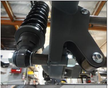
The threaded side goes down as shown. Install the provided spacer up against the back of the axle bracket.
