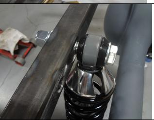
You can now install the coil-overs using the provided 5/8" hardware. One washer goes against the bolt head and the other goes against the nylock.
