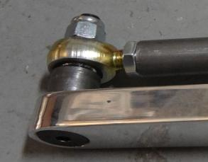
The flat head bolt goes in from the outside to match the taper of the countersunk end of the aluminum arm.
