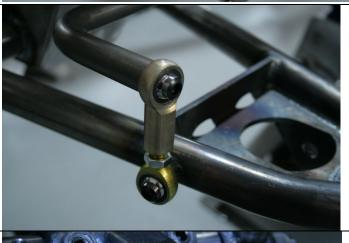
Assemble the male and female heims with the jam nut. Install the female rod end on the anti-sway bar using the provided machined button head bolt. Install the male rod end on the lower control arm using the provided machined button head bolt.
