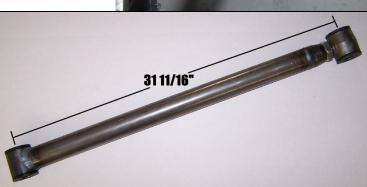
Adjust all the 4-link bars to 31 11/16" center to center and tighten the jam nuts.
