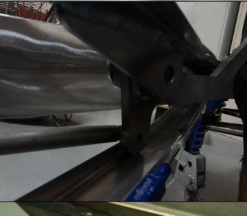
Insert the pivot pin into the bottom of the brake pedal arm
