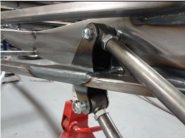
Install the 4-link bars with the adjuster side onto the frame using the provided 5/8" hardware. The upper bolt goes in from the inside and the lower bolt goes in from the outside as shown.
