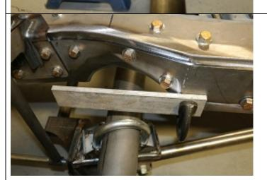
We now need to center the axle. We placed a couple scrap pieces of aluminum as straight edges and clamped them in place. It doesn't matter much where you place them on the frame so long as they are mounted the same on both sides.
