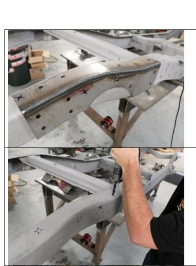
Place the C-Notch plate onto the frame at the axle centerline. There are 4 existing holes on the frame that line up with the new plate but they are too small so we will need to drill them out to 7/16". Use a sharpie and mark one of the holes (we chose the front/top hole) for alignment.
