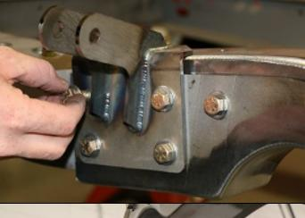
Install the 4 side bolts through the shock bracket and tighten.
