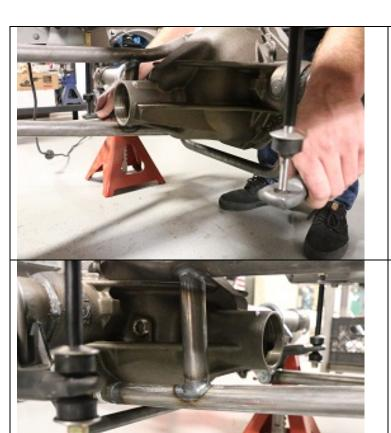
With the top bushing and cupped washer in place you can now lift the anti-sway bar up into place making sure the studs line up with the holes on the bar.
