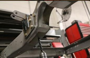
Drill the remaining holes using the C-Notch plates as a template including the ones underneath.
