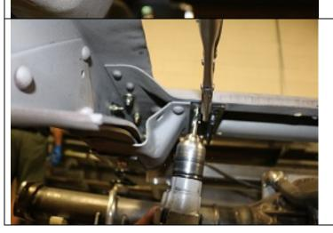
Place a vise grip or c-clamp on the bracket to hold it in place. Drill the remaining 3 holes and install hardware loosely.
