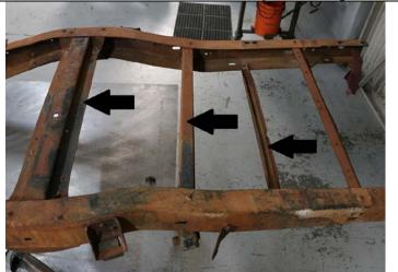
There are 3 crossmembers at the rear portion of the frame that are relevant to this installation.
