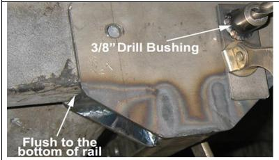
With the channel bracket pressed flush against the frame rail, use a 3/8 drill bit and drill the two outside holes in each frame rail using the holes in the channel bracket as a guide.
