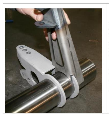
The axle brackets are designed to slide over a 3 inch axle tube before the bearing flange housings are installed. If the bearing ends are already on the axle bracket 3 inch ribs can be cut 90 degrees to the flat shock mounting face and re-attached after the bracket is tacked on. The brackets are positioned 44 1/8 centers for stock width and 40 1/8 for the 2 inch mini-tub. The flat rear surface of the axle bracket is parallel with the front mounting surface of the 3<sup>rd</sup> member.
