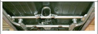
If the optional sub-frame connectors and driveshaft loop were purchased they are installed next. The driveshaft loop cross-member is installed under the brackets on the connectors using the  $3/8 \times 1$  inch bolts, nuts and washers. Center the loop in the driveshaft tunnel before tightening.
