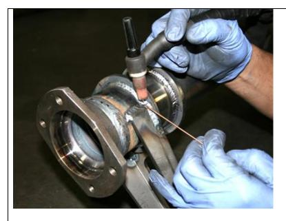
Finish welding the axle brackets and the panard bar bracket as pictured. If an <u>optional</u> sway bar is being used the sway bar brackets are located on the front of the axle tubes at axle centerline on 33 inch centers.
