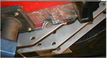
The flange on the outer rail will have to have a radius for clearance to install the link bolt if the top hole is to be used. The bracket shown is for a two inch inset mini-tub application.
