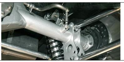
The sway bar is connected to the axle housing brackets with a  $3/8 \times 1^{1/4}$  inch button headed bolts. The link is tapped 3/8 inch left and right for ease of adjustment while still bolted up. The sway-bar end uses a lock washer and the bracket on the axle housing a nylock nut.
