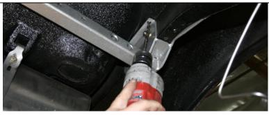
Using the 5/16 inch holes on the flange of the channel bracket as a guide, use a long shank 5/16 drill bit and drill the 4 holes (2 on 68-69) through the floor of the trunk.
