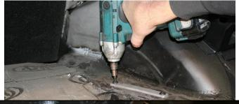
Install the 4 hole re-enforcing plate (2 hole on 68-69) over the holes and install the  $5/16 \times 24 \times 1^{1/4}$  inch button head bolts and washers through the plate, trunk sheet metal and through the cross-member channel bracket.
