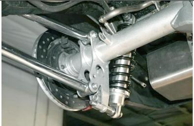
Next the rear axle assembly has to be installed. It's a lot easier to install the bare housing and install the  $3^{\rm rd}$  member, axles and brakes later but that's your choice. First, install the coil-over's on the front of the top cross-member using the  $5/8 \times 18 \times 4\frac{1}{2}$  bolt, washer on each side of the shock bushing then the 5/8" spacer against the cross-member and the full nylock nut on the back.
