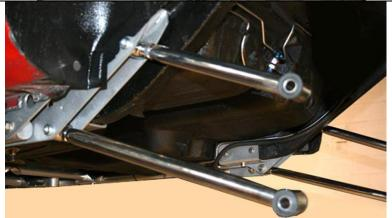
Mount the 4-link bars into the frame bracket using the button headed  $5/8 \times 18 \times 2\%$  bolts with the stainless adjustors forward in the frame bracket. Tighten the ½ nylock nuts and position bars to accept rear axle housing.
