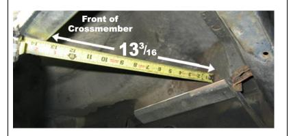
Next using the 5/16 inch bracket holes as a guide, drill one 5/16 hole through the floor pan and install one of the  $5/16 \times 1\frac{1}{4} \times 24$  button head bolts and install nut on inside and tighten. This will keep the bracket from moving around while drilling and all holes will line up when finished. Finish drilling remainder of the holes using a long shank 5/16 inch drill bit.
