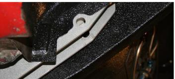
The flange on the outer rail will have to have a radius for clearance to install the top link bolt for the 4-link bar.
