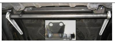
The optional 7/8 inch billet sway bar is installed in the sway bar housing using the sleeve bushings, next the flat washer then the splined aluminum arms are installed. Clock the arms evenly and tighten clinch bolts. The sway bar housing is bolted the back side of the cross-member using four  $5/8 \times 18 \times 2^{1/2}$  inch bolts and full nylock nuts.
