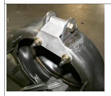
The torque arm tabs are welded on by using the supplied fixture tool. Bolt fixture to the lowest 2 third member bolts flat against the housing flange. Bolt on the two supplied tabs using the  $\frac{1}{2}$  by  $3\frac{1}{2}$  inch bolt and with the longer tab to the passenger side of the housing. Bottom of tabs may need sanding to fit. Weld outside and wrap welds also to the inside.
