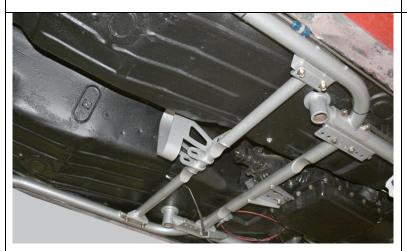
The Torque Arm cross-member is installed with the driveshaft loop facing rearward and the end flanges of the cross-member under the brackets on the subframe connectors. Using the 3/8 x 16 x 1 inch bolts and washers, bolt the cross-member to the sub-frame brackets and install the 3/8 Nylock nuts and washers. Double check to make sure that the driveshaft loop is centered in the driveshaft tunnel before final tightening.
