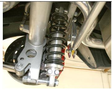
The photo on the left shows the panard bar attached to the axle housing bracket using  $\frac{1}{2}$  x 20 x 2 inch bolt, washers and Nylock nut. The process is repeated on the right side on the panard bar bracket that is bolted to the coil-over cross-member. The three hole adjustment gives the choice of raising or lowering the rear roll center.
