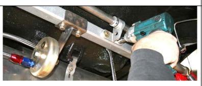
When installing the <u>optional</u> ¾ inch rear sway bar, first slide the lock rings on. Next the split urethane bushing with flange facing lock ring. Next the brackets with the flange facing rearward and the sway bar forward. Leave lock rings loose to facilitate install. Install the four 3/8 x 2½ bolts, washers and Nylock nuts. Adjust sway bar location after rear axle is installed. Note: We mounted the fuel filter and pump to the cross-member.
