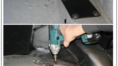
Install the 4 hole re-enforcing plate (2 hole on 68-69) over the holes and install the  $5/16 \times 24 \times 1^{1/4}$  inch button head bolts and washers through the plate, trunk sheet metal and through the cross-member channel bracket.
