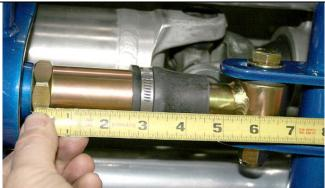
The slider shaft travels in and out very little but still needs to be positioned in the slots 6¼ inches from the back of the wrench flats on the housing to the center of the sleeve with the bushing in it. This adjustment allows the slider shaft to be in the middle of its travel. Tighten the Nylock nut.
