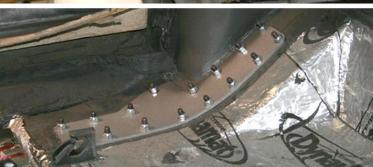
Next using the 5/16 inch bracket holes as a guide, drill one 5/16 hole through the floor pan and install one of the  $5/16 \times 1^{1/4} \times 24$  button head bolts and install nut on inside and tighten. This will keep the bracket from moving around while drilling and all holes will line up when finished. Finish drilling remainder of the holes using a long shank 5/16 inch drill bit.
