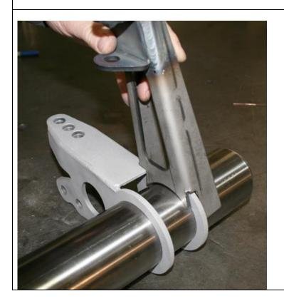
The axle brackets are designed to slide over a 3 inch axle tube before the bearing flange housings are installed. If the bearing ends are already on the axle bracket 3 inch ribs can be cut 90 degrees to the flat shock mounting face and re-attached after the bracket is tacked on. The brackets are positioned 44 1/8 centers for stock width and 40 1/8 for the 2 inch mini-tub.
