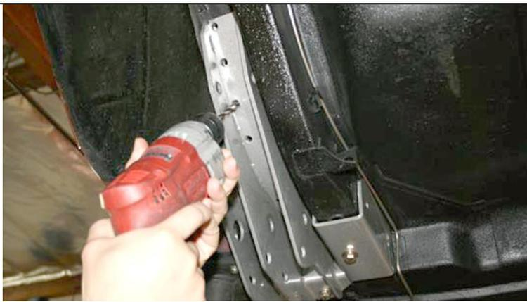
Next using the 5/16 inch bracket holes as a guide, drill one 5/16 hole through the floor pan and install one of the 5/16 x 1 1/4 x 24 button head bolts and install nut on inside and tighten. This will keep the bracket from moving around while drilling and all holes will line up when finished. Finish drilling remainder of the holes using a long shank 5/16 inch drill bit.
