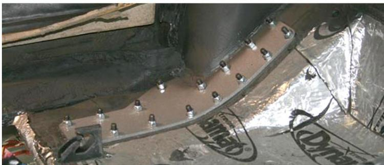
Align the appropriate curved re-enforcing plate on the inside of the car over the drilled bolt holes and have a second person push the 5/16 button headed bolts through the bracket underneath. Install the washers and the 5/16 Nylock nuts and tighten.
