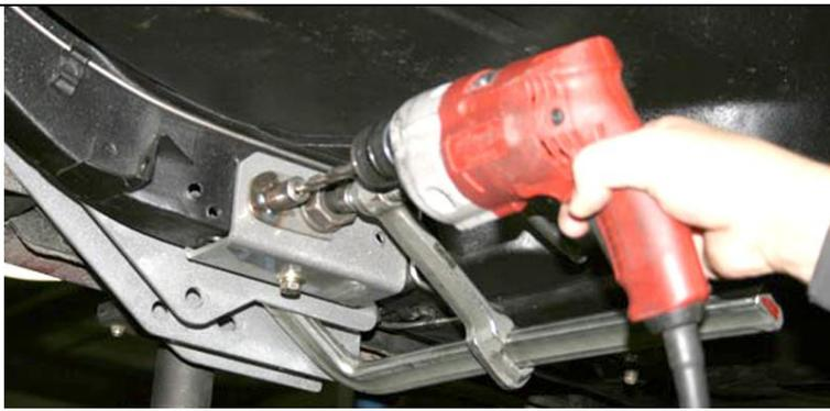
Using a 3/8 inch drill bit and using the 3/8 inch holes in the channel bracket, drill the inside holes through the frame rail. Then using the furnished drill guide, align the drill bit in the guide with the drill bit in the previously drilled hole and clamp the guide as pictured. This will facilitate in keeping the drill bit in line with the outside holes in the bracket.
