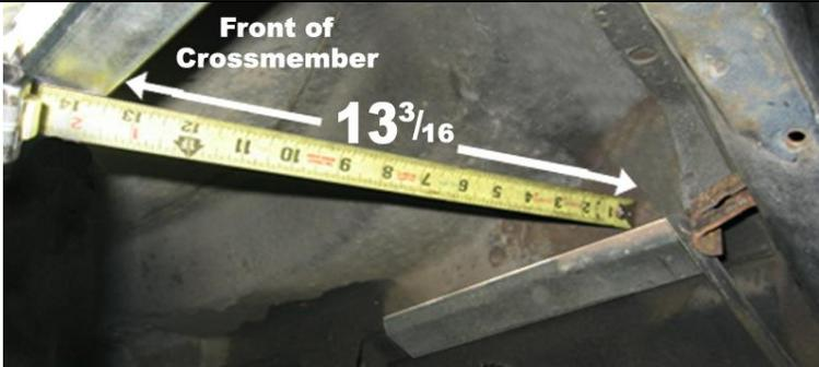
The coil-over cross-member is next. Remove any hanger brackets that will interfere.
