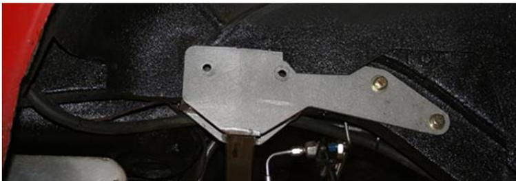
The 1968-69 Camaro coil-over cross-member is located by the two existing 3/8 x 16 threaded holes in the frame rail. Using the four 3/8 x 16 x 1 inch bolts, fasten the front flange of the cross-member to the frame and push the saddle of the cross-member flush before tightening.
