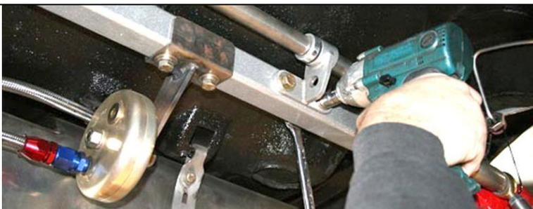
When installing the optional ¾ inch rear sway bar, first slide the lock rings on. Next the split urethane bushing with flange facing lock ring. Next the brackets with the flange facing rearward and the sway bar forward. Leave lock rings loose to facilitate install. Install the four 3/8 x 2½ bolts, washers and Nylock nuts. Adjust sway bar location after rear axle is installed. Note: We mounted the fuel filter and pump to the cross-member.
