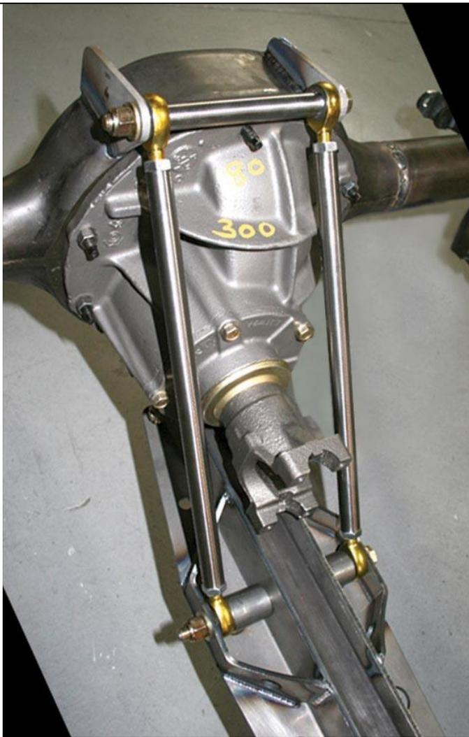
The pinion support tubes have left and right hand rod ends to facilitate pinion angle adjustment. Adjust the tubes to approximately the same length with an equal amount of threads showing on each rod end. Install the tubes with the right hand rod ends on the inside of the top brackets using the  $\frac{1}{2}$  by 8 inch bolt, washers, 5.2 inch spacer in between rod ends and Nylock nut.
