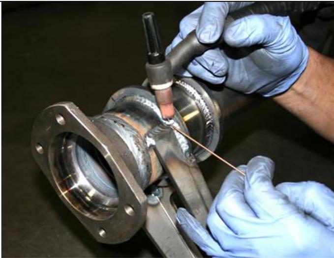
Finish welding the axle brackets and the panard bar bracket as pictured. If an optional sway bar is being used the sway bar brackets are located on the front of the axle tubes at axle centerline on 33 inch centers.
