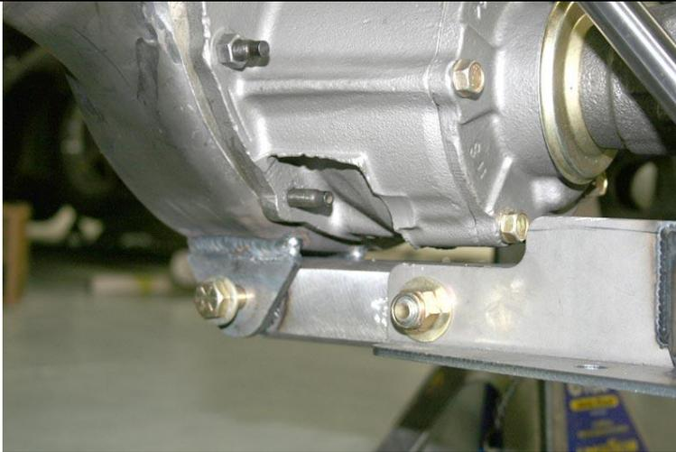
**Install the rear of the Torque Arm to the tabs on the bottom of the rear end housing using a 1/2 inch by 3 1/2 inch bolt, washers and nut. Lightly tighten.**
