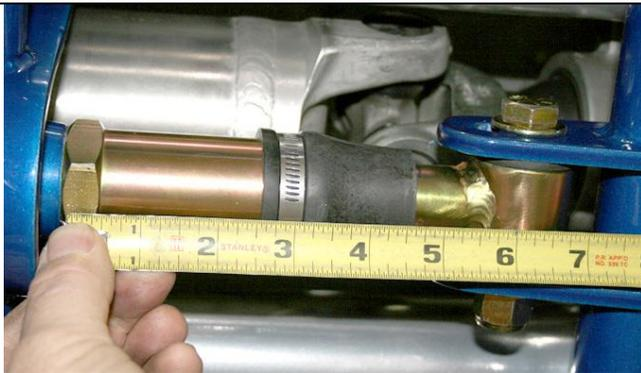
The slider shaft travels in and out very little but still needs to be positioned in the slots  $6\frac{1}{4}$  inches from the back of the wrench flats on the housing to the center of the sleeve with the bushing in it. This adjustment allows the slider shaft to be in the middle of its travel. Tighten the Nylock nut.
