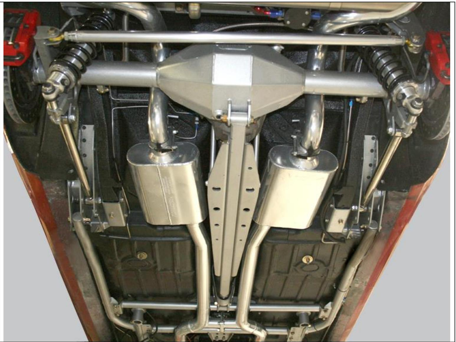
**The Torque Arm rear suspension completely installed. The TCI Camaro uses 2½ inch exhaust system and Flowmaster mufflers. Everything is tucked up close and tight so installing the driveshaft should be done before installing exhaust system and leaving one of the pinion support tubes off until the driveshaft is installed.**
