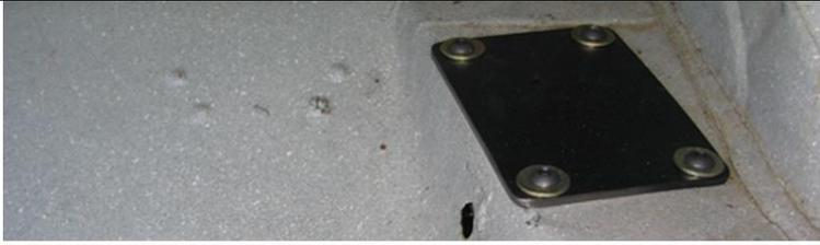
Install the 4 hole re-enforcing plate (2 hole on 68-69) over the holes and install the 5/16 x 24 x 1¼ inch button head bolts and washers through the plate, trunk sheet metal and through the cross-member channel bracket.
