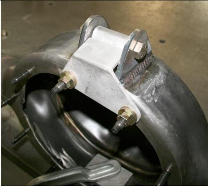
The torque arm tabs are welded on by using the supplied fixture tool. Bolt fixture to the lowest 2 third member bolts flat against the housing flange. Bolt on the two supplied tabs using the  $\frac{1}{2}$  by  $3\frac{1}{2}$  inch bolt and with the longer tab to the passenger side of the housing. Bottom of tabs may need sanding to fit. Weld outside and wrap welds also to the inside.
