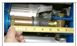
The slider shaft travels in and out very little but still needs to be positioned in the slots 6¼ inches from the back of the wrench flats on the housing to the center of the sleeve with the bushing in it. This adjustment allows the slider shaft to be in the middle of its travel. Tighten the Nylock nut.
