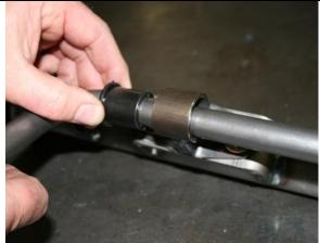
Slide the urethane bushings on and hand press the bushings into the tube brackets.
