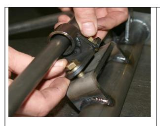
Assemble the sway bar by sliding the tube brackets onto the ends of the bar, then bolt the tube brackets to the cross member using the four 3/8 by 1 inch bolts, washers outside and the nut on the inside of the sway bar bracket on the cross member. This has to be done first before the bushings are installed because the clearance between the bar and the bracket is to close with the bushing installed.
