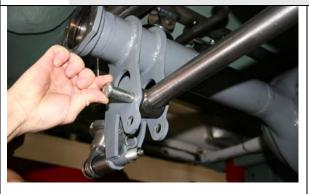
Install the trailing arm bars using the 5/8 by 2¾ inch button head bolts and the half nylocs in the top holes in the axle brackets (street), lower hole for strip application.
