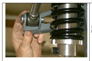
Install the panhard bar next using the 9/16 by  $2\frac{1}{4}$  inch button head bolts and the half nyloc nuts.
