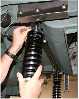
Install the coil-over shocks (250 lb. rate) on the cross member with the  $\frac{1}{2}$  by 2 3/8 inch button head bolt, washers and half nyloc nuts.
