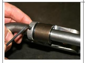
Center the bar on the cross member and slide the aluminum rings on the sway bar with set screws installed up against the urethane bushing flange, and tighten set screws.
