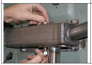
Install the front four ½ by 4 inch bolts, washers and nuts through the cross member and the frame channels.
