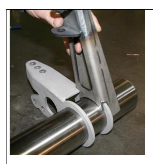
The panhard bar bracket is installed onto the back of the driver's side axle bracket with the channel facing out and the inner curved radius inside the outer axle bracket rib up against the 3 in axle tube rotated down against the rear face of the axle bracket.
