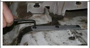
Tighten the 3 button head bolts on the inner frame sub-frame support plates that were left loose. This will pull the connectors up tight against the frame.
