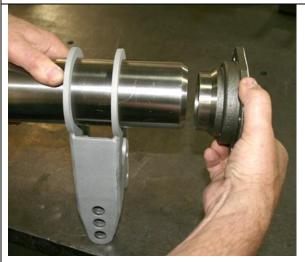
The rear axle brackets, panhard bracket and the sway bar brackets are installed as per the drawing. I would highly recommend getting this done by somebody with experience narrowing rear axle housings. The kit uses a nine inch <u>centered pinion</u> axle housing. Recommended axle bracket installation is to slide the brackets over the axle tubes without the bearing flanges attached rather than cut the brackets and re-weld together on the housing.
