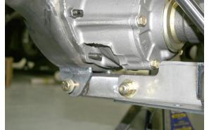
Install the rear of the Torque Arm to the tabs on the bottom of the rear end housing using a  $\frac{1}{2}$  inch by  $3\frac{1}{2}$  inch bolt, washers and nut. Lightly tighten.
