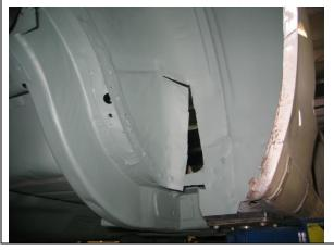
We started by cutting a pie shaped piece out in the seat belt bracket area. Then we slit the wheel well in the center and worked that section inward toward the frame. Keep working it until it is flat like the rear section of the wheel well. We then filled the pie cuts, welded everything up and did a little hammer work. It was a little extra body work but it allowed us to put a 285-40-18 tire on a 9.5 inch wide rim. Looks awesome and the car sits low with a lot of rubber on the ground.
