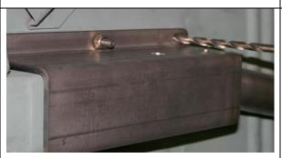
After drilling the first hole, install one of the 5/16 button head bolts through the drilled hole and tighten. This helps in drilling the remaining holes.
