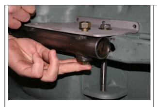
The sub-frame connectors (L&R) are installed by bolting the rear hole of the connector with a ½ inch by 3½ inch bolt to the rear hole in the support plates to locate the front channel in the correct location before drilling holes.
