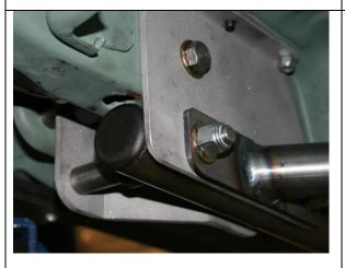
Install the plastic end cap on the end of the sub-frame connector tube by tapping with a hammer after paint or powder coating. Tapering the front ribs on a sander makes installation easier.
