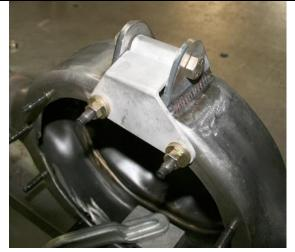
The torque arm tabs are welded on by using the supplied fixture tool. Bolt fixture to the lowest 2 third member bolts flat against the housing flange. Bolt on the two supplied tabs using the  $\frac{1}{2}$  by  $\frac{3}{2}$  inch bolt and with the longer tab to the passenger side of the housing. Bottom of tabs may need sanding to fit. Weld outside and wrap welds also to the inside.
