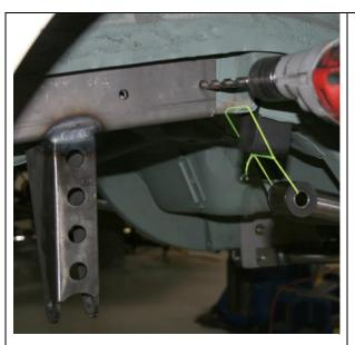
Next the 3/8 inch holes in the sides of the channel brackets need to be drill out. The front holes on both sets of brackets can be drilled from the inside and the outside without using the drill guide plate. Drill the outside holes both sides and the front inside holes from the inside.
