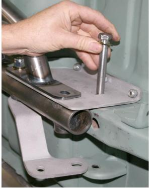
The long  $6\frac{1}{2}$  inch bolt previously installed in the support plate needs to be unbolted and partially pulled out to allow the brace bracket to be rotated into the proper location.
