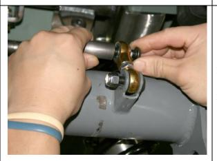
Install the rod end links on the sway bar using the 3/8 by  $1\frac{1}{4}$  inch button head bolt and lock washer. Bolt the bottom of the link to the sway bar bracket on the housing.
