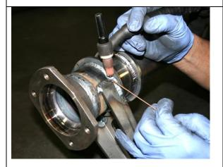
Finish welding axle brackets and panhard bar bracket the full 360 degrees inside and outside.
