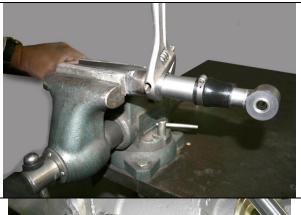
The Torque Arm is shipped with the slider assembly separate to facilitate packaging. The slider has been pre-assembled with Teflon bushings and has been installed in the Torque Arm to check for proper fit. We use anti-seize on the threads to prevent galling. When painting or powder coating the assembly, tape the threads on the slider and plug the hole in the Torque Arm tube.
