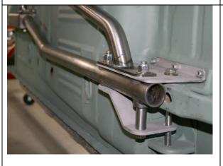
The trailing arm will be installed either in the top hole (stock spring location), street application or the bottom hole, strip application. On this project, we are using the street setup. Install the ½ by 5½ inch bolt through the brace, through the 1¾ inch long spacer, through the sub-frame connector, support plate and through the stiffener flange rear hole. Install nut and washer and leave loose.
