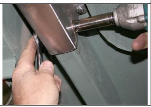
Next, install the rear 3/8 by 2½ inch bolt through the channel bracket and tighten.
