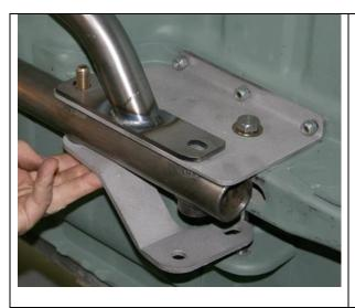
Push the two rear connector ½ by 3½ inch bolts through the front holes of the stiffener flanges, install nuts and washers and leave loose.
