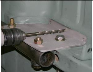
The three holes in the rear inner sub-frame support plate that was bolted on earlier are drilled next with a long 5/16 inch drill bit. I would still use the "install one bolt then drill remaining holes procedure".
