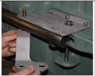
Installation of the torque arm cross member/frame stiffener is next. Remove the two ½ by 3½ inch bolts fastening the rear of the sub-frame connectors to the support plates. Install one of the bolts and washers through the front of the trailing arm brace brackets (L&R) then through the sub-frame connector then partially through the support plate. Let the rear of the plate hang down temporally. Do both sides.
