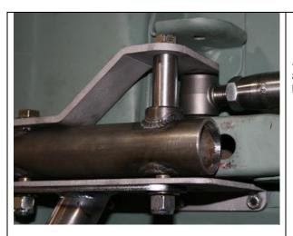
Adjust the trailing arm to 20 1/8 inch centers for a starting point. Install the adjustor end of the trailing arm between the stock inner spring pocket and the brace.
