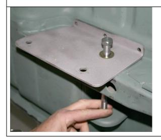
With all the old suspension removed, start by installing the rear inner subframe support plates (L&R) aligned with the front stock leaf spring hole using the  $\frac{1}{2}$  inch by  $\frac{6}{2}$  inch bolts, washers and nuts that are furnished and lightly tighten.
