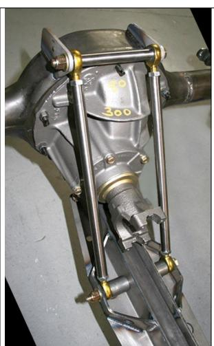
The pinion support tubes have left and right hand rod ends to facilitate pinion angle adjustment. Adjust the tubes to approximately the same length with an equal amount of threads showing on each rod end. Install the tubes with the right hand rod ends on the inside of the top brackets using the ½ by 8 inch bolt, washers, 5.2 inch spacer in between rod ends and Nylock nut.
