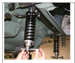
Install the 5/8 by 6 inch bolt with washer on the shock and  $1\frac{3}{4}$  inch spacer on the bolt.
