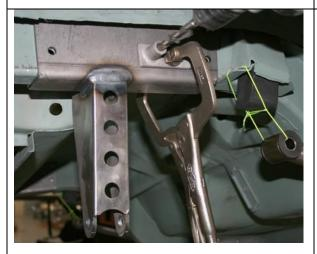
Using the drill guide plate (furnished), center over the drilled 3/8 inch holes (#2 then #3) on the outside of the frame, securely clamp and drill through existing hole then the frame rail on the other side and then through the existing hole on the inside of the channel bracket. Be patient and hold onto the drill motor as the drill bit will grab when it goes through the inside rail and tries to go out the channel bracket hole.
