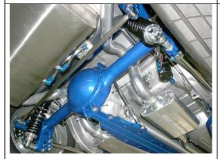
Using a straight edge on the both the housing flanges, measure to the edge of the snubber housings to center housing and adjust panhard bar as needed.
