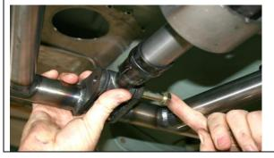
With the heavy lifting done, bolt the front of the Torque Arm slider shaft to the cross member center bracket with the slots using the ½ by 3 inch bolt, washers and nut.
