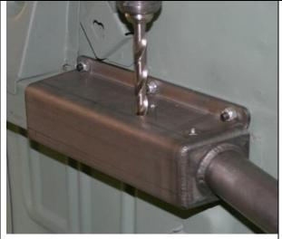
Next, the eight ½ inch front side holes in the front sub-frame connector channel have to be drilled in the frame. To keep the holes centers straight, drill from the inside and outside of the rail rather than try to drill all the way through from one side. Hold the drill securely as it will want to grab the thin frame sheet metal.
