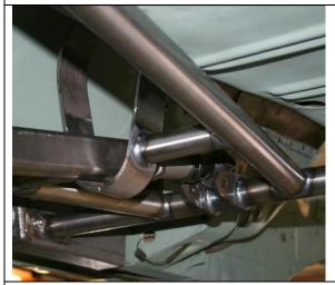
Slide the axle assembly under the car and rest the Torque Arm slider assembly in the driveshaft loop.
