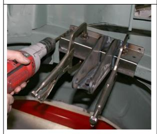
Clamp channel firmly against the rail and so that it remains in place while you are drilling the four 5/16 inch holes per channel through the floor. Again use the "install one bolt and drill remaining holes procedure". Repeat drilling process for the driver's side channel bracket.
