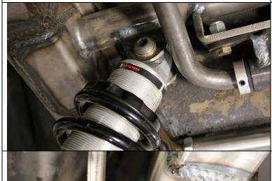
Install the coil-over shocks with the threaded end onto the cross member with the ½ by 2 3/8 inch button head bolt, washers and half nyloc nuts. We placed the adjuster on the bottom inside for ease of adjustment.
