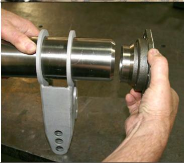
The rear axle brackets, panhard bracket and the sway bar brackets are installed as per the drawing(below). I would highly recommend getting this done by somebody with experience narrowing rear axle housings. The kit requires the use of a <u>centered pinion</u> axle housing with 3" axle tubes. Recommended axle bracket installation is to slide the brackets over the axle tubes without the bearing flanges attached rather than cut the brackets and re-weld together on the housing.
