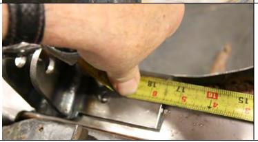
The driver side bracket also installs onto the frame 17.5" forward of the stock leaf spring hanger hole.
