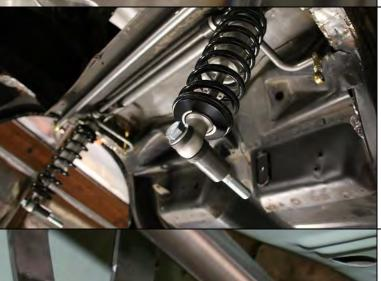
Install the 5/8 by 6 inch bolt with washer on the shock and 1¾ inch spacer on the bolt.
