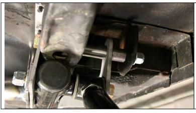
Install the plastic end cap on the end of the sub-frame connector tube by tapping with a hammer after paint or powder coating. Tapering the front ribs on a sander makes installation easier.
