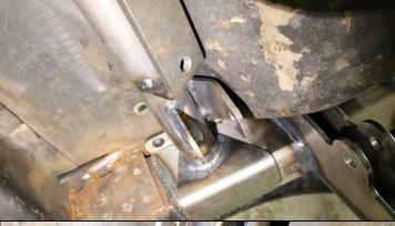
You can now install the crossmember back into place. It should be a tight fit. Same thing as before. It needs to be tight up against the frame and as far back as possible.
