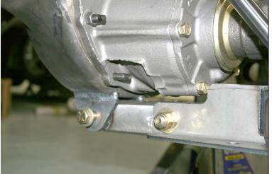
Install the rear of the Torque Arm to the tabs on the bottom of the rear end housing using a ½ inch by 3½ inch bolt, washers and nut. Lightly tighten.
