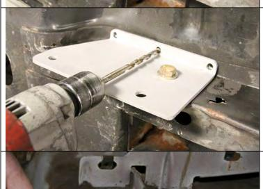
Push the plate flat up against the floor and drill three 5/16 inch holes up through the plate and into the floor.
