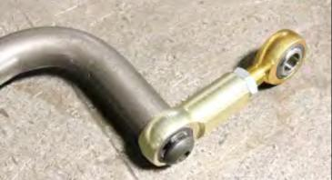
Install the female side of the heim joint onto the sway bar using the button head bolts.
