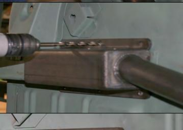
With the sub-frame channel pushed solidly against the floor and the rear of the connector bolted to the support plates, drill the first hole through the floor with a 5/16 drill bit using the channel's holes as a guide pattern.
