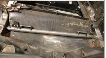
The coilover crossmember needs to be test fit between the rails.
