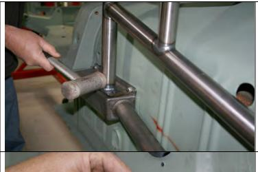
Lift the torque arm cross member/frame stiffener up between the rails; with the drive shaft loop up against the floor. Tap cross member into place between the sub-frame channels.
