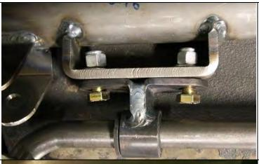
Install the anti-sway bar onto the crossmember with the arms hanging down freely. Tighten the bolts.
