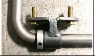
Slide the locking rings on and leave loose at this time.
