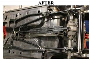
With all the old suspension removed, start by installing the rear inner sub-frame support plates (L&R) aligned with the front stock leaf spring hole using the ½ inch by 3½ inch bolts, washers and nuts that are furnished and lightly tighten.
