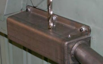
Next, the front sub-frame connector channels have to be drilled in the frame. To keep the holes centers straight, drill from the inside and outside of the rail rather than try to drill all the way through from one side. Hold the drill securely as it will want to grab the thin frame sheet metal.
