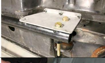
The sub-frame connectors (L&R) are installed by bolting the rear hole of the connector with a ½ inch by 5½ inch bolt. Leave the bolt loose for now. The lower bolt will have to be removed a few steps down.
