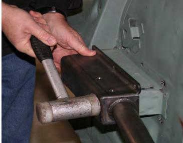
Tap the sub-frame connector front channel over the stock frame rail until flush with the floor. Note: You may have to do a little hammer work on the stock frame rails to square them up to install channels. The rails on our '67 Mustang had taken quite a beating during the last 40 years.
