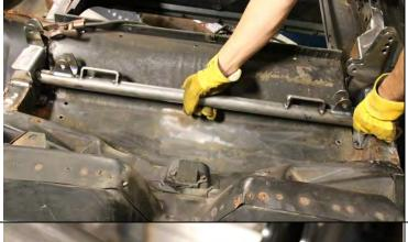
Remove the crossmember carefully from the center making sure it comes out evenly. It should be a tight fit. Take your time. Once you get a little space between the frame and plate it will be easier to pry from there. Just make sure it comes out evenly or else the frame plates will move on the crossmember.
