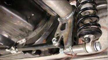
Install the trailing arm bars using the 5/8 by  $2\frac{3}{4}$  inch button head bolts and the half nylocs
