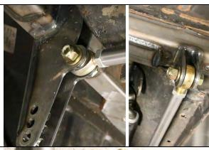
Install the frame stiffener bar into the upper hole on the passenger side and the only hole on the driver side. Make adjustments on the heims until the bolts install easily.
