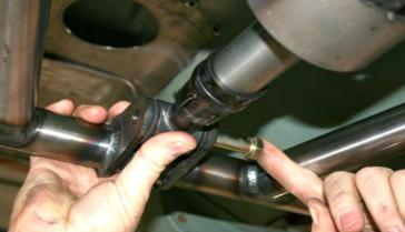
With the heavy lifting done, bolt the front of the Torque Arm slider shaft to the cross member center bracket with the slots using the ½ by 3 inch bolt, washers and nut. \*Do not tighten down yet
