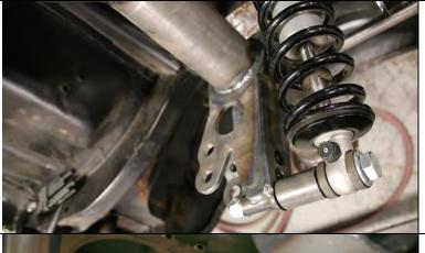
Time to install the axle housing assembly. You can use a hydraulic floor jack under the third member or have a couple of your strong friends, like I did, lift the ends of the housing while I pushed the long 5/8 inch bolts through the lower mounting hole in the axle brackets. I left off the axles and brake kit because of the extra weight. Tighten the 5/8 nyloc nuts.
