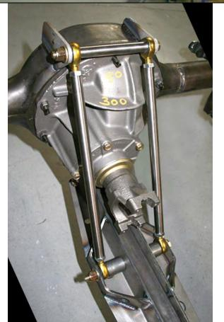
The pinion support tubes have left and right hand rod ends to facilitate pinion angle adjustment. Adjust the tubes to approximately the same length with an equal amount of threads showing on each rod end. Install the tubes with the right hand rod ends on the inside of the top brackets using the ½ by 8 inch bolt, washers, 5.2 inch spacer in between rod ends and Nylock nut.
