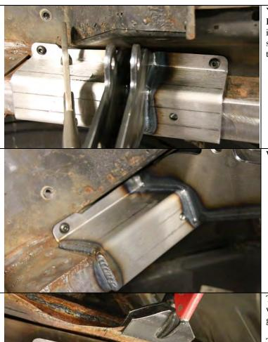
You can now install the two 5/16 inch bolts up through the floor. Because there is usually no carpet in this area of the trunk you can install these bolts from the bottom or from the top. There is no sandwich plate for these. Tighten the bolts to bring the frame bracket tight up against the frame rail.
