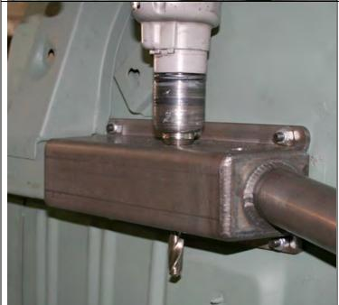
Afterward you can run the drill through both holes to ensure the bolts will go through clean. Hang onto the drill; it will want to grab the frame sheet metal.
