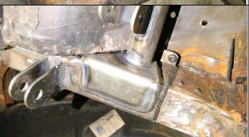
Complete welding the frame plate onto the frame brackets.
