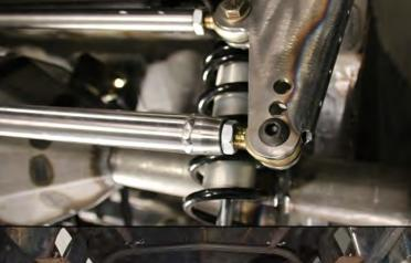
Install the panhard bar on to the frame bracket using the 1/2 by  $2\frac{1}{4}$  inch button head bolts and the half nyloc nuts.
