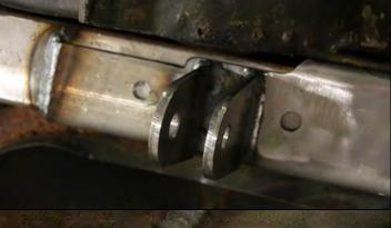
Weld the bracket to the frame only, not to the trunk sheet metal.
