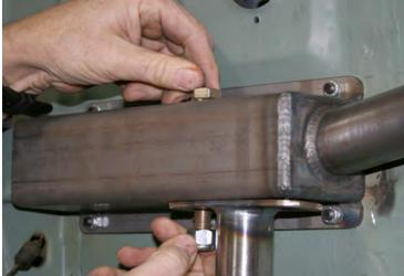
Install the front four ½ by 4 inch bolts, washers and nuts through the cross member and the frame channels.
