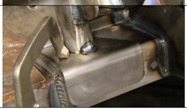
You can now remove the passenger side coilover to gain access for the passenger side tack weld. Same thing here, get a good tack. If at all possible try to put two on opposing sides of the round tube.
