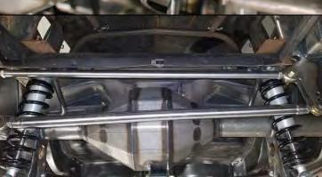
Adjust the panhard bar as needed to center the housing at ride height.
