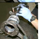
The sway bar brackets are located on the front of the axle tubes(see drawing above) at axle centerline on 32.75 centers. Finish welding sway bar brackets and straighten rear housing.
