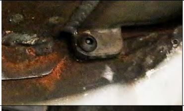
With the bracket clamped securely in place you can drill the one 5/16" hole up through the floor.
