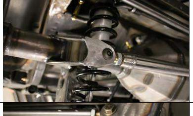
Install the panhard bar on to the axle bracket using the 1/2 by  $2\frac{1}{4}$  inch button head bolts and the half nyloc nuts.
