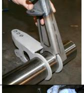
The panhard bar bracket is installed onto the back of the driver's side axle bracket with the channel facing out and the inner curved radius inside the outer axle bracket rib up against the 3 in axle tube rotated down against the rear face of the axle bracket.
