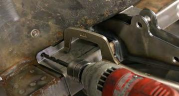
With the bracket clamped securely in place you can begin drilling the 5/16" holes up through the floor.
