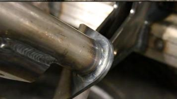
Once we had removed our crossmember we put a couple more tack welds on each side and reinstalled it. This was to confirm that the plates hadn't moved out of place.
