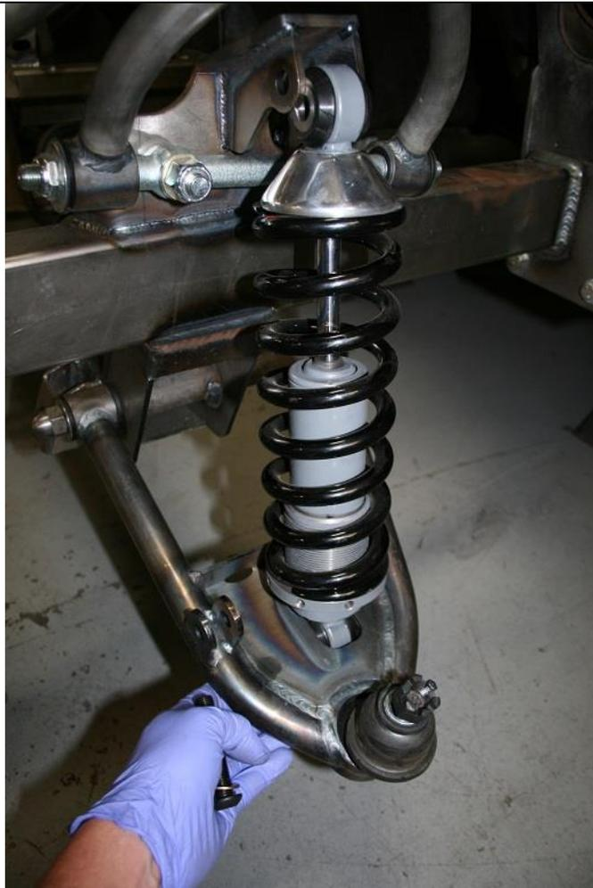
Once the lower shock bolt is tight you can now lift the control arm up into place and install the upper shock bolt.
