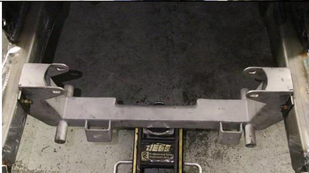
Slide the cross member (steering rack brackets forward) between the rails behind (firewall side) the locating plates.
