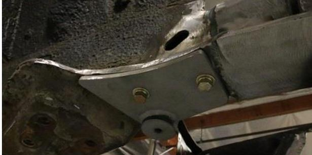
The sway bar brackets are mounted using existing holes on the frame.
