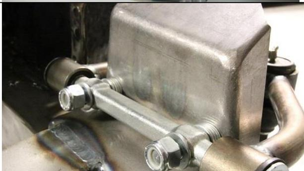
**Install the upper a-arm with the shaft on the inside of the tower. Install one washer on the button head bolt and push it through the tower from the outside. Install 4 camber adjustment washers, the crossshaft, and one additional washer. Put some anti-seize on the threads and install the nylock. Position the a-arm bolts in the center of the caster slots for a starting point and tighten the nuts.**
