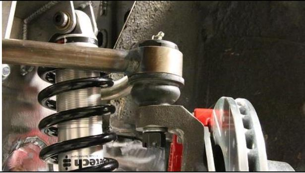
Install the top a-arm ball joint into the spindle. Install AN washer and nut. Tighten and cotter pin.
