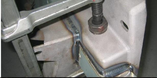
Use a C-clamp from the inside and pull the bracket down snug to the top of the frame rail.
