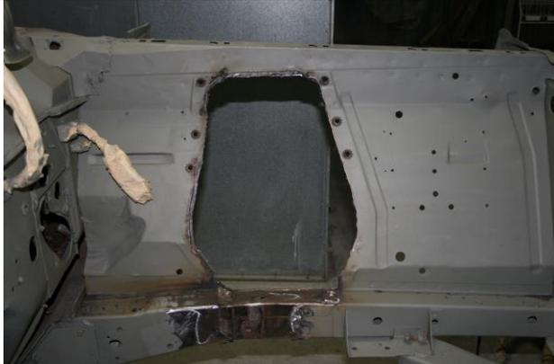
Remove the shock tower. You can now grind down the 1/4" extra we left all around. Grind it back flush to the stock panel being careful not to grind back too far.
