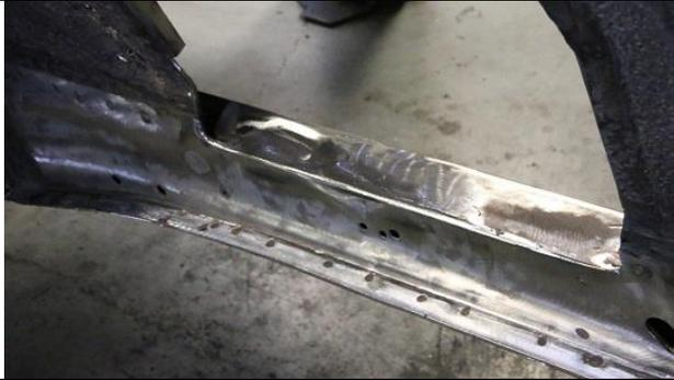
**Grind the welded area flat and square.**
