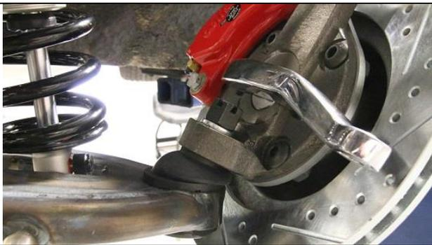
The spindle and brake assemblies come completely assembled with the bearings packed and seals installed. With the steering arm forward and caliper rearward set the spindle onto the lower ball joint and install AN washer and nut, tighten and cotter pin.
