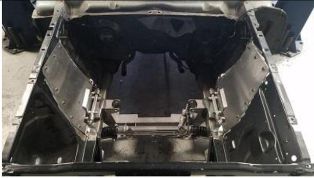
Proper ride height is set with the lower a-arm level to the ground. Adjust the height with the threaded ring on the bottom of the coil-over.
