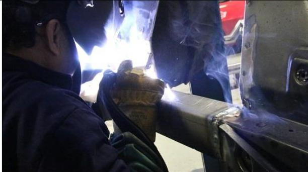
**It's time to tack weld the inner and outer boxing plates to each other and to the frame. When it comes to welding, we prefer to heli-arc because it's cleaner and less grinding afterwards but a wire feed will work fine, just a little more clean-up grinding afterwards.**
