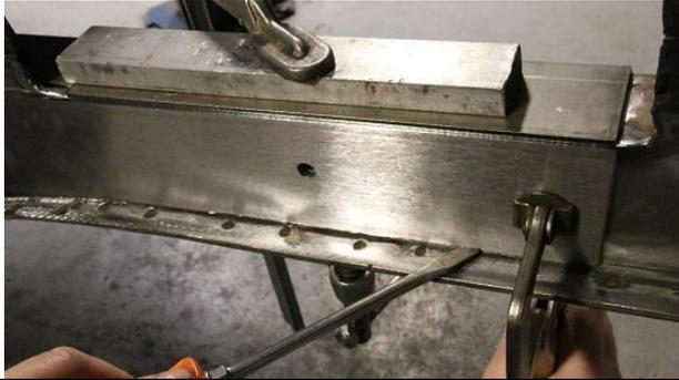
**Install a couple clamps, one to hold the side plates and one to hold the top plate. The gap along the top edge is critical. Align the boxing plate edges parallel with the top plate exposing an even section of the stock frame that when welded will tie both boxing plates to each other and to the frame.**
