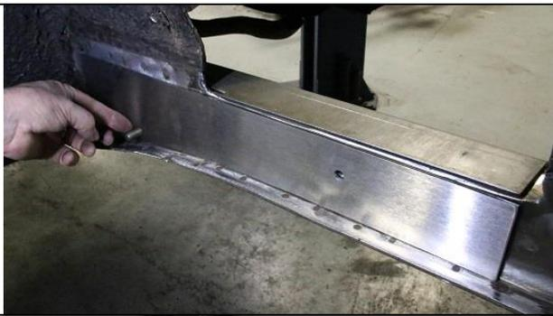
**You can now install the inside plate using the same rear bolt hole to locate it. Install the nut and tighten it down.**
