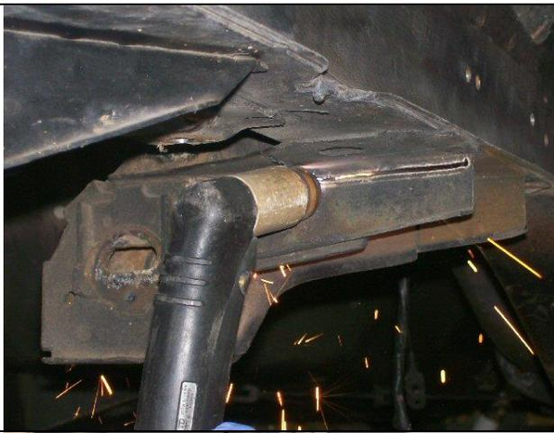
**Remove the lower A-arm/motor mount brackets first.**
