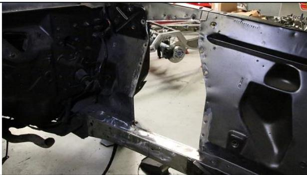
**Preparing the frame rails. Remove all excess material, welds and paint from the main rails for the installation of the boxing plates.**
