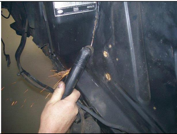
The vertical cuts on the towers are made at the bend radius between the tower and fender panel.
