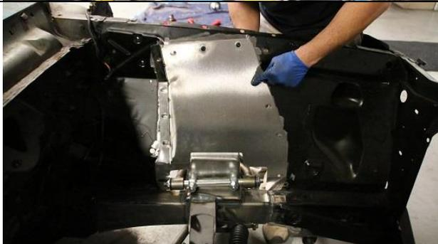
**Position the correct panel over the a-arm until the pre-existing factory bolt holes line up. Most of the top holes in the panel use existing factory holes.**
