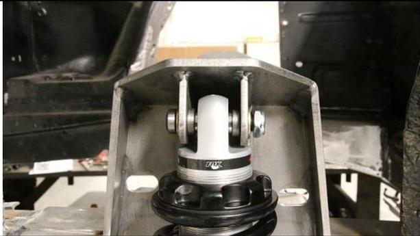
**The shock assembly is installed next using the 1/2 inch bolts. The threaded adjuster side of the shock goes on the top. Install the 1/2" bolt from the front using the provided, spacers, AN washers and short nylock and tighten.**
