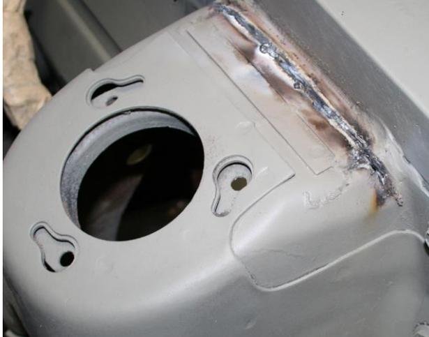
**When removing the inner fenderwells cut across the top leaving roughly 1/4" gap at the fender. This will be ground back before the panels go in.**
