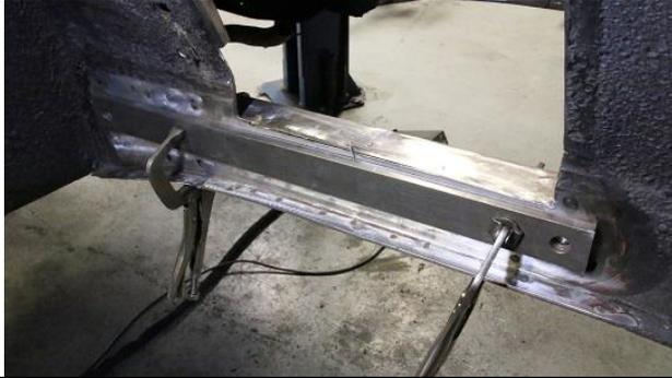
**We made a quick little welding guide fixture so we could weld the seam as straight as possible. We clamped a two foot flat piece of material just below the top of the frame rail to maintain a straight edge. Then we just laid the welding tip onto the top of the bar and used it as a guide.**
