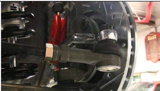
**Install the jam nut and tie rod end onto the inner tie rod. Then install the tie rod end onto the steering arm, install the castle nut, tighten it down and insert the cotter pin.**
