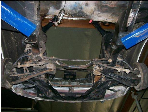
Remove all the old suspension components including the steering column.
