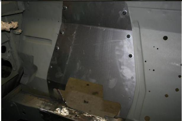
You will need to install the panels at this point to use them as a template to finish cutting the lower portion of the factory panel. There are existing holes you can use to hold it in place. Use the provided 5/16" hardware to hold them in place.
