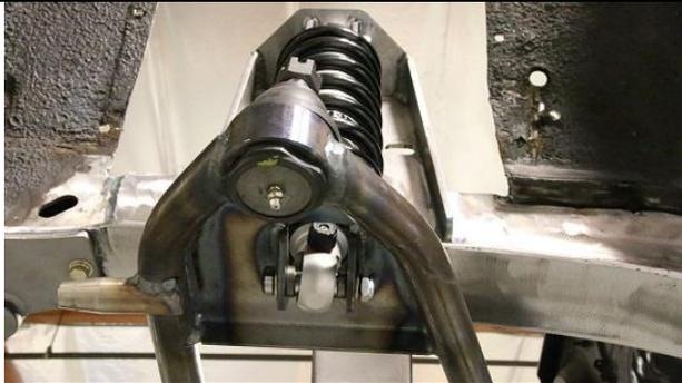
**The adjuster knob should point outwards towards the ball joint. Install the 1/2" bolt from the front using the provided, spacers, AN washers and short nylock and tighten.**
