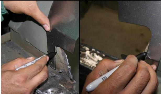
Make a mark on the factory panel using the new inner panel as a template. Remove the panel and cut along the line.
