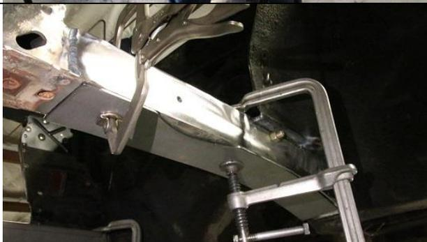
**Lay the bottom boxing plate on the bottom of the frame with the rounded cutout to the outside. The leading edge of the bottom plate will need to sit flush with the rear edge of the factory anti-sway bar mount.**
