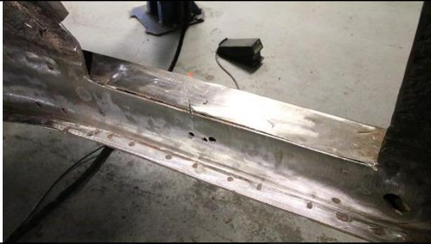
**There is a split between the top and side rails that need to be massaged down. Any high spots or irregularities that aren't straight or square must be removed.**
