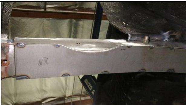
Using the rounded cutout of the lower boxing plate as the template, grind the stock frame flange until they match the profile of the boxing plate edge.
