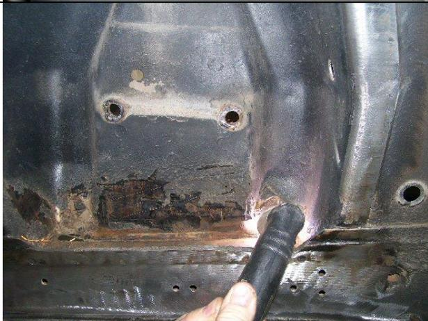
**Next are the shock towers. The first cut will be made from inside the wheel well just above the main frame rail flange.**
