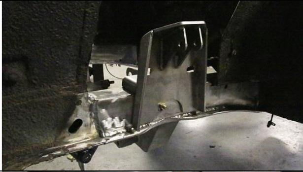
The a-arm/shock tower bracket is mounted with the highest a-arm bolt slot forward and the lowest slot rearward. This is the built in anti-dive feature.
