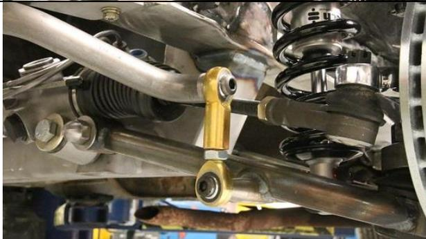
**Install the 1/2" rod ends as shown with the male end facing up. The sway bar rod end link needs to be straight up and down to allow adequate rack and pinion tie rod lock to lock clearance. Adjust the bar positioning by sliding it for and aft and side to side then tighten the bracket bolts.**
