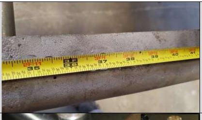
Make a mark at 37" on both passenger and driver side frame rails. Draw a line across the top of the frame rail at 37". This is done so that we can find the center of the frame rail from side to side. That way the crossmember is centered in the chassis.
