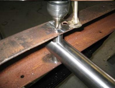
Install the cross member between the rails with the shock tubes parallel to the ground and facing forward.
