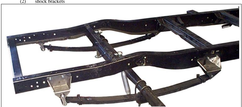
\*NOTE\* Before removing the stock leaf springs, mark the frame and take measurement as to where the stock axle centerline was. The frame needs to be at the typical 2 degrees rake to mimic actual ride height. Keep the frame at this rake throughout the installation.
