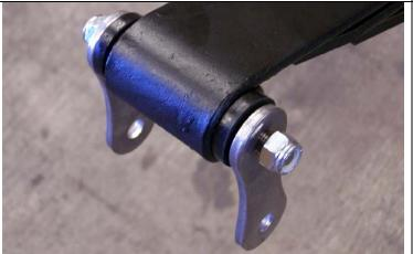
Place the shackle bushings into the rear spring eyes. Slide the shackle pins through the bushings. Place the dogbones onto the shackle pins and install the nylocks.
