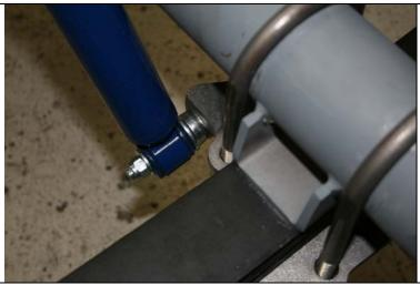
Fasten the shock studs to the 5-holes plate with ½-20 nylock and washers. Attach the shocks and fasten with the provided nylocks, stainless steel cupped washers and flat washers.
