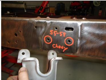
To remove the rivets holding the brackets, grind the rivet heads flush. Center punch the rivet and drill through using progressively larger drills up to a 5/16" drill. Take care not to drill the original rivet holes larger or off center, as you will be locating your new brackets with these holes.
