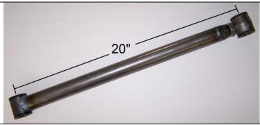
Adjust all the 4-link bars to 20" center to center and tighten the jam nuts.
