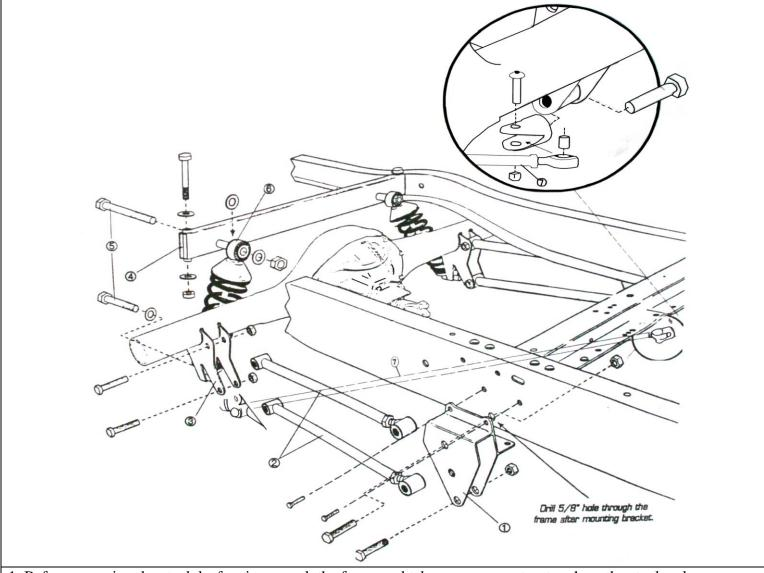
1. Before removing the stock leaf springs, mark the frame and take measurement as to where the stock axle centerline was. The frame needs to be at the typical 2 degrees rake to mimic actual ride height. Keep the frame at this rake throughout the installation. Remove the brake lines, driveshaft, leaf springs, rearend, rear leaf hangers etc.
