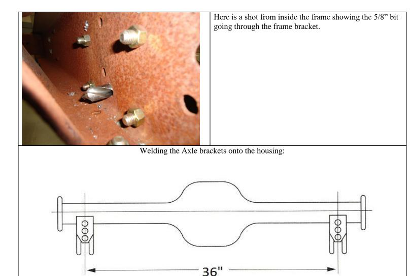
The factory leaf spring pads must first be removed from the housing and the area cleaned up. The axle brackets are installed at 36" Center to center. Make sure that they are centered on the housing. Also, make sure the pinion is pointed up one degree in comparison to the flat area at the backside of the brackets (where the three holes for the coil-overs are located). Use the 3<sup>rd</sup> member mounting face on a Ford 9" or the differential cover on a GM housing as reference.
