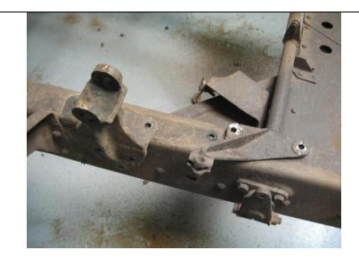
Start by removing the front stock spring hangers and e-brake cable bracket. To remove the rivets holding the brackets, grind the rivet heads flush. Center punch the rivet and drill through using progressively larger drills up to a 5/16" drill. The rivet should be relatively easy to punch out. If it is not, then continue drilling with a 3/8" drill. Take care not to drill the original rivet holes larger or off center, as you will be locating your now parts with these holes.
