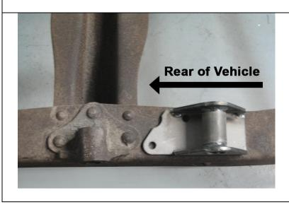
Remove the stock rear shackle bracket rivets in the same manner as the front spring hanger bracket rivets. The shackle brackets are positioned on the rails with the welded side on the inside of the rail. Line up the brackets with the holes of the original brackets. It may be necessary to align-drill a couple of these holes. Use three  $3/8-16 \times 1-1/4$  bolts, nuts, and one washer under each nut to fasten each bracket. The square front edge of the bracket faces to the front of the vehicle.
