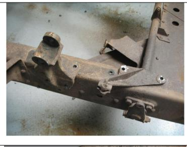
Start by removing the front stock spring hangers and e-brake cable bracket. To remove the rivets holding the brackets, grind the rivet heads flush. Center punch the rivet and drill through using progressively larger drills up to a 5/16" drill. The rivet should be relatively easy to punch out. If it is not, then continue drilling with a 3/8" drill. Take care not to drill the original rivet holes larger or off center, as you will be locating your now parts with these holes.
