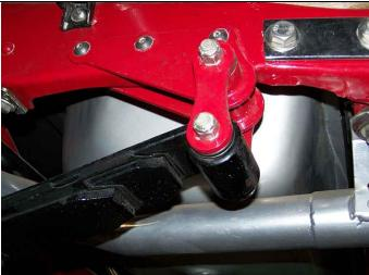
\*NOTE\* Leave the leaf spring disconnected from this attachment point at this time.
