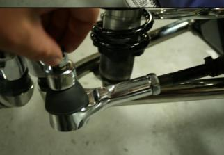
Install the jam nut and outer tie rod end onto both sides of the rack. With the rotors pointing straight ahead(0 toe) install the tie rod ends into the bottom of the steering arm. Torque the tie rod ends to 60 ft. lbs. and install the cotter pin.
