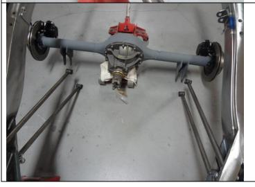
Place the rear axle onto a jack and roll it under the frame just behind the Link bars
