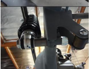
\*NOTE\* Installing the optional Ridetech adjustable shocks.
