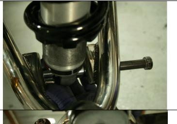
The lower shock bolt also holds the anti-sway bar heim joint. Install the bolt from the back going forward. There will be two ½" spacers that will go on either side of the shock head between the control arm tabs. There is one more spacer to be installed once the bolt is in place.
