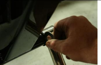
Place the 3rd washer in between the bushing and the pin as shown.
