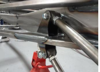
Install the 4-link bars with the adjuster side onto the frame using the provided 5/8" hardware. The upper bolt goes in from the inside and the lower bolt goes in from the outside as shown.
