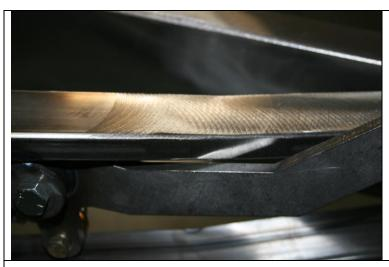
Leave the jam nut loose. Final adjustment will be done once the body is installed and carpet is in place.
