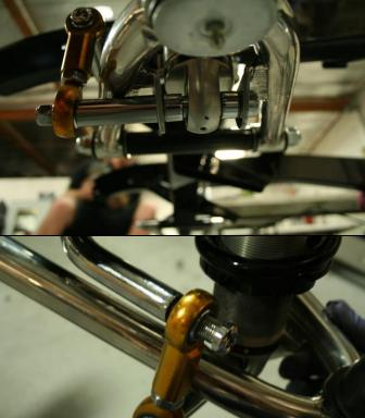
Once the special bolt and spacers are installed you can now attach the anti-sway bar rod ends.
