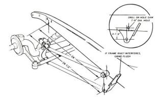
frame bracket. Upper hole is located 4 7/8" above lower hole and 24" back from lower fender brace hole on frame.
